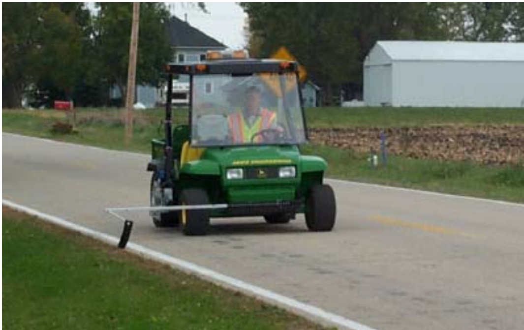
Figure C.6. Ames Engineering lightweight inertial profiler operation.
