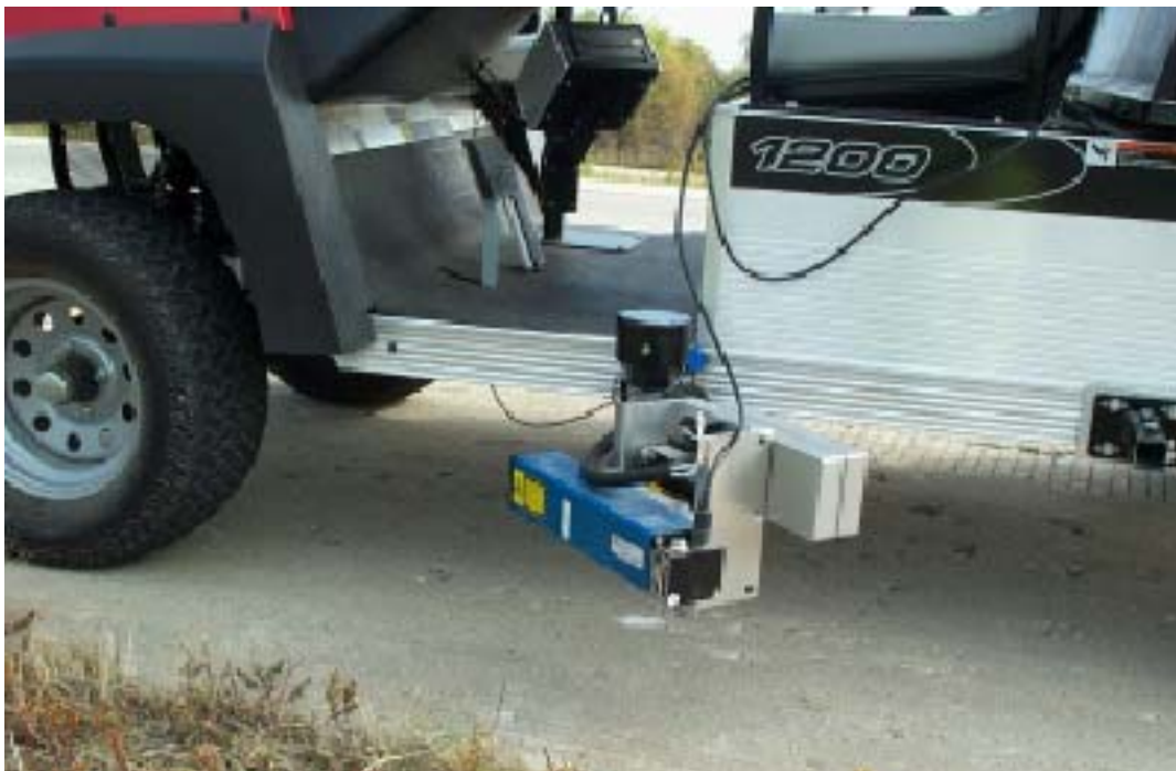
Figure C.4. SSI lightweight inertial profiler, sensor arrangement.
