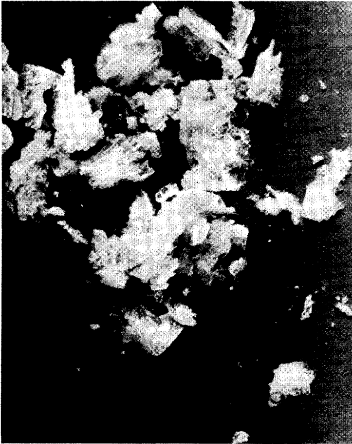
Fig. 7. Platelike debris collected from modeling fixture during Regime III wax simulation.
