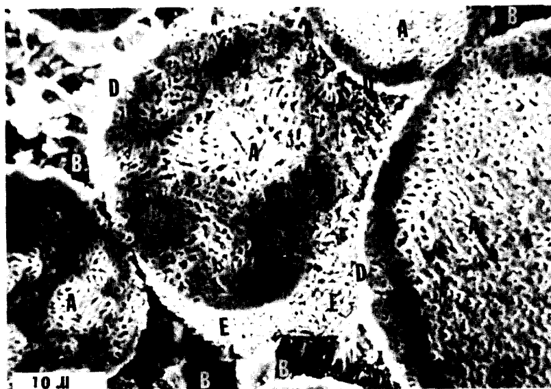
FIG. 7. A scanning electron photomicrograph of a 15% gold-containing amalgam surface after being polished mechanically and etched in this order, first using Wing's double cyanide solutions [8] and then using a 30% nitric acid solution. Dark pits (marked B ) show that \gamma_1 phase is removed by the nitric acid etchant. White rings marked D and boundary regions of \gamma grains marked E both correspond to Au-Sn phase.
