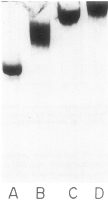
FIG. 4. Native polyacrylamide gel electrophoresis performed on 5% slabs according to Nelles et al. (23) of \alpha_2 M-trypsin complex and its PEG derivatives. Five to seven micrograms of each protein sample was applied. Gel A—unmodified \alpha_2 M—trypsin complex; gel B—PEG-2 derivative; gel C—PEG-4 derivative; gel D—PEG-20 derivative. The direction of migration is from top to bottom with the bottom being the anode.
