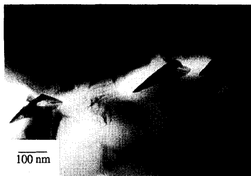
Fig. 5. M_7X_3 precipitates on grain boundary in B + C-doped alloy. Alloy received anneal of 1473 K for 20 min.
