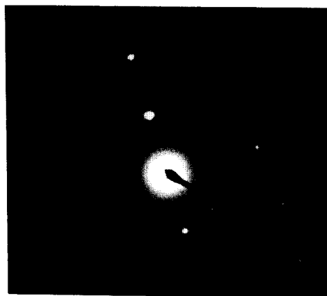
Fig. 1. Selected area diffraction pattern for \text{Cr}_7\text{C}_3 in C-doped alloy that was annealed (1373 K, 20 min) and heat treated (973 K, 100 h).
