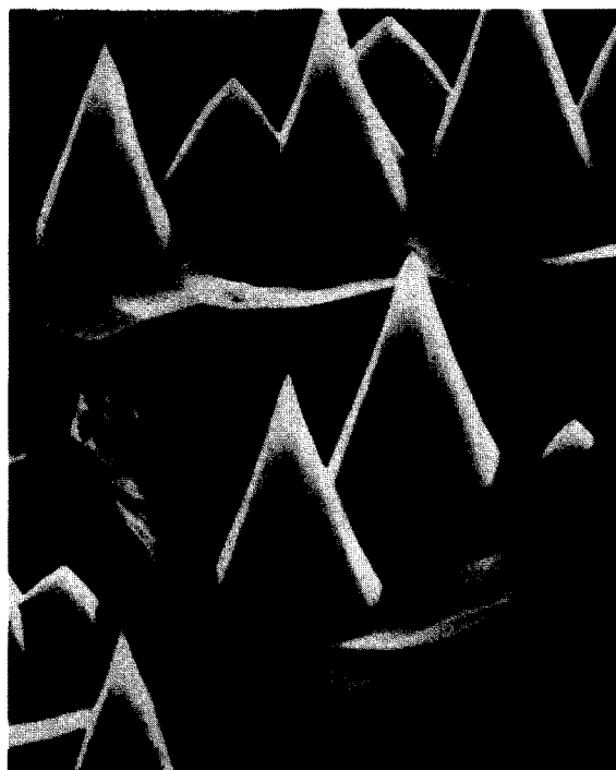
Fig. 3. Scanning electron micrograph of an \langle 11\bar{3}1 \rangle Ni-8% Cu alloy after bombardment with 40 keV \text{Ar}^+ to 2 \times 10^{19} ions/cm 2 showing how the octagonal pyramids originate in the centre of the pits. Magnification 6000 \times .
