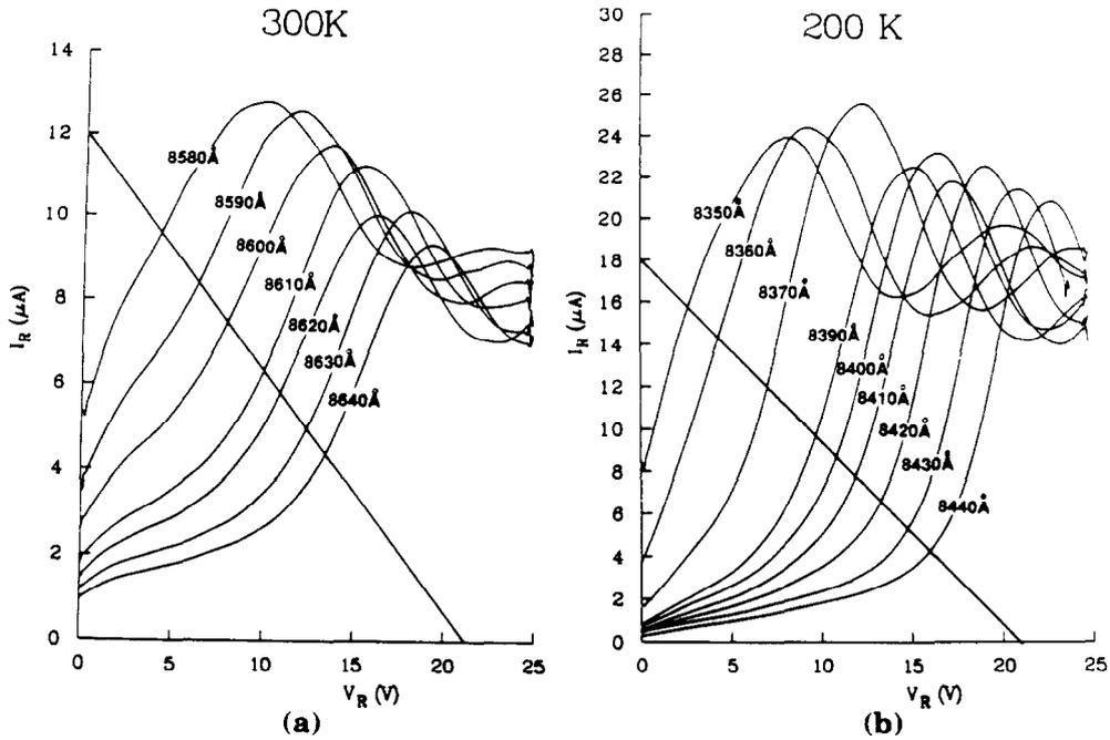
**Figure 1** Measured photocurrent-voltage characteristics at various wavelengths in a p-i(MQW)-n photodiode (a) at 300 K and (b) at 200 K.
