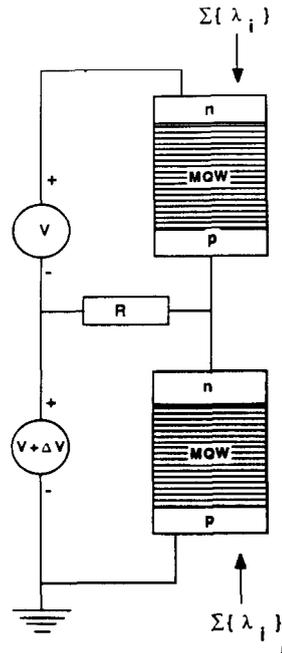
**Figure 2** Schematic for photocurrent subtraction using two diodes for wavelength selective detection. The potential developed across the resistance  $R$  is proportional to the differential photocurrent.
