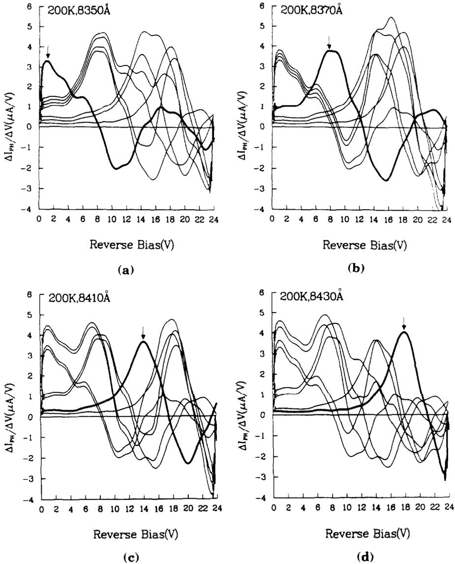
Figure 3 Values of  $\Delta I_{ph} / \Delta V$  at 200 K for different states of 4 channels  $\lambda_j$ . The bold current represents the ON state of  $\lambda_i$  only when  $\lambda_1 = 8350 \text{ \AA}$  (a),  $8370 \text{ \AA}$  (b),  $8410 \text{ \AA}$  (c), and  $8430 \text{ \AA}$  (d).
