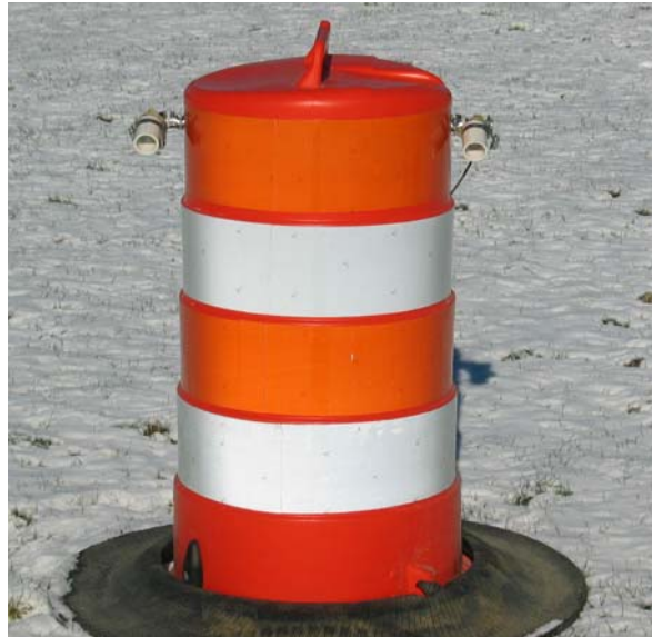
Figure 12. Pyroelectric Detectors on a barrel
