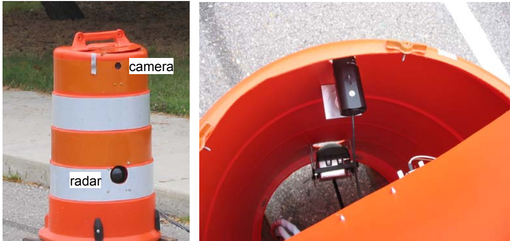
Figure 20. Reference system barrel with video and radar
