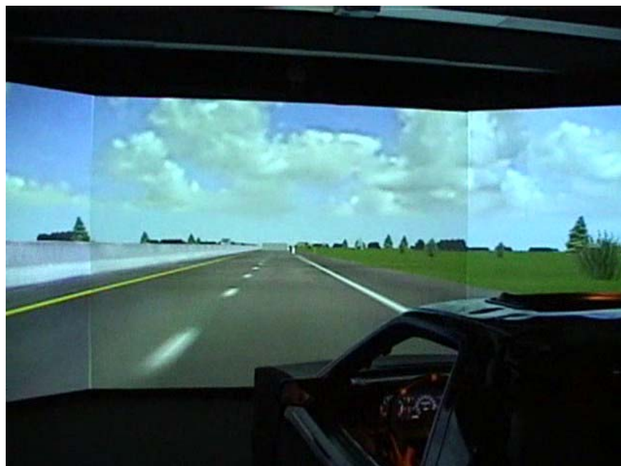
View of simulator-controlled roadway on which post-mounted warning lights advised drivers to decrease their speed when approaching stopped traffic.
