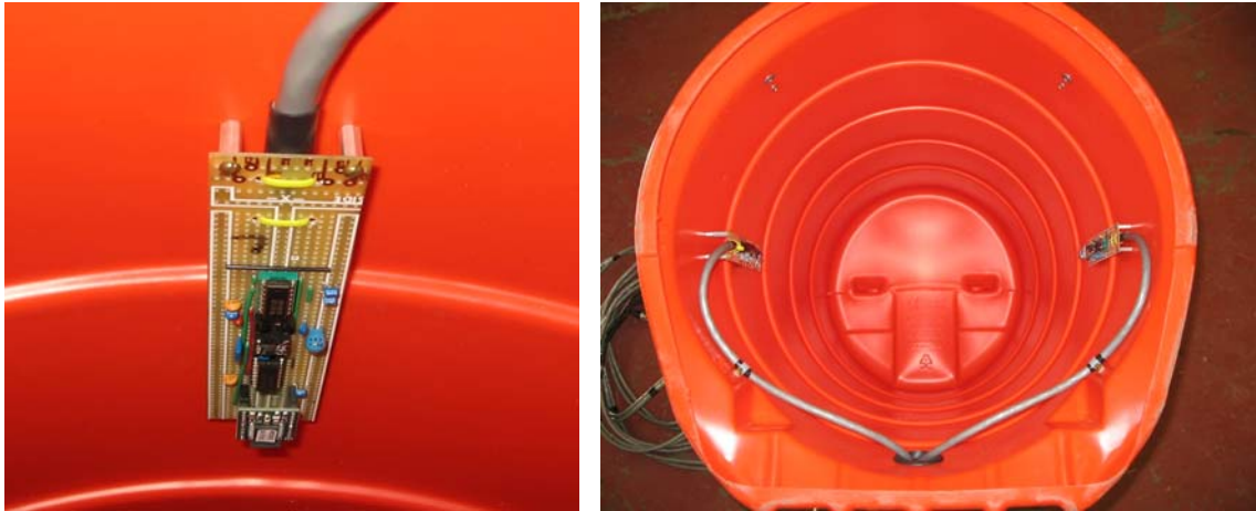
Figure 14. Magnetometers mounted inside a barrel.
