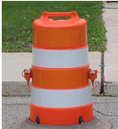
Figure 17. Photoelectric sensors mounted to barrel
