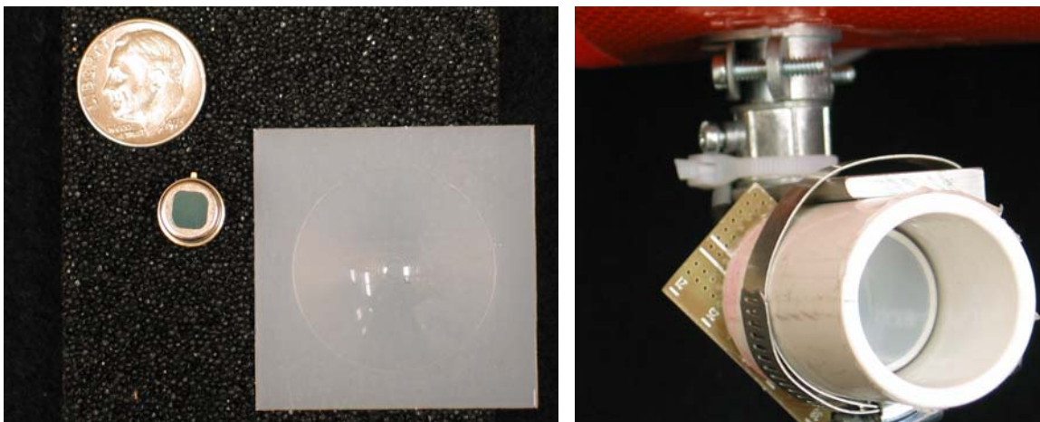
Figure 10. Pyroelectric detector and fresnel lens and assembled sensor
