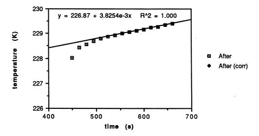
Note that each measurement will have two line fits associated with it: a "before" and an "after" line. The three graphs (original, before, and after) are printed and retained for reference later. The extrapolated lines and resultant "initial" and "final" temperatures are shown below:
