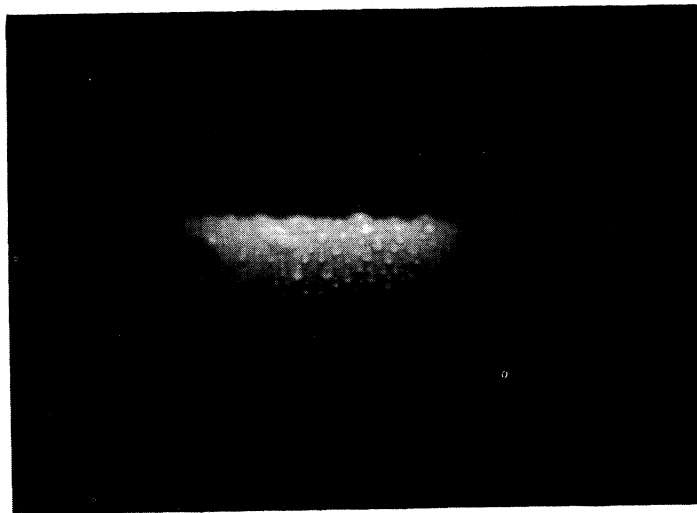
FIGURE 6— DROPWISE CONDENSATION OF SUPERHEATED STEAM
