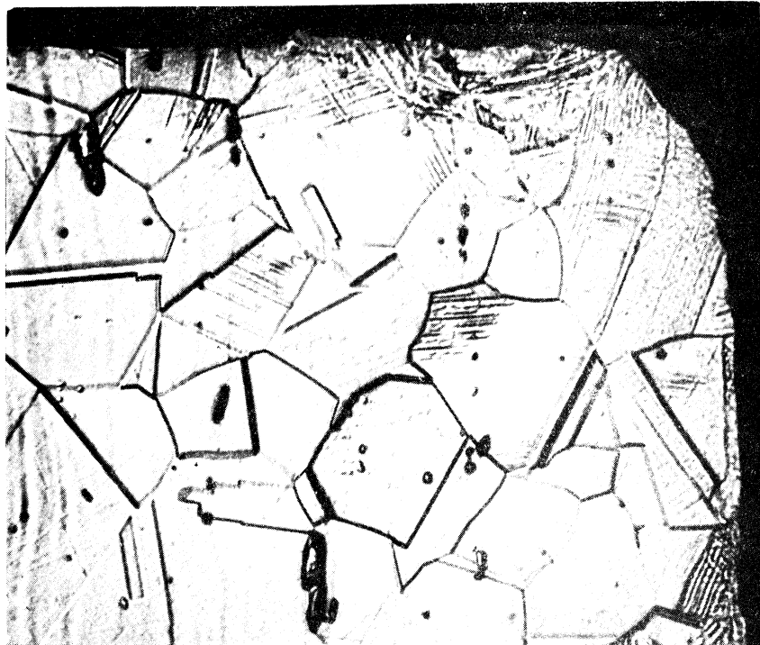
Figure 22. Microsection illustrating the "rounding" of a samples edge. Stainless steel specimen #26. Standard cavitation. Throat velocity 97.2 fps. 12 hours test duration in water. Etched. 1000X.
