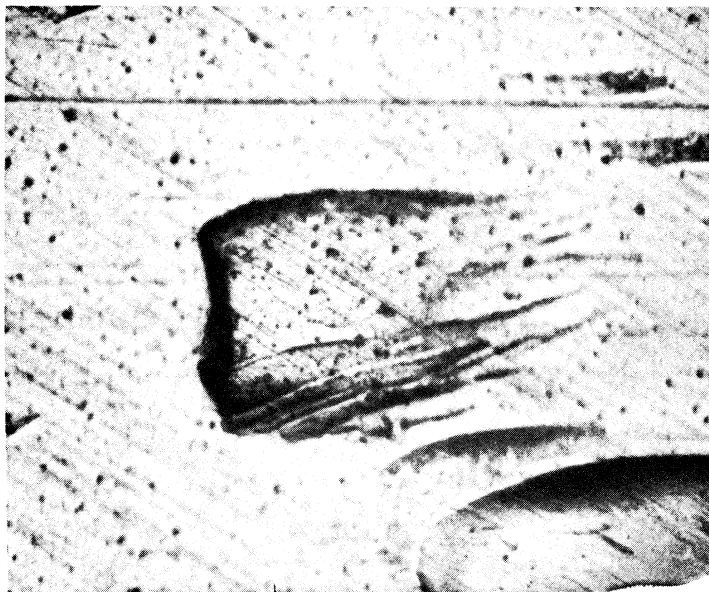
Figure 20. Macrograph showing small pits on the bottom of a large shallow crater. Same sample as shown in Figure 19.
