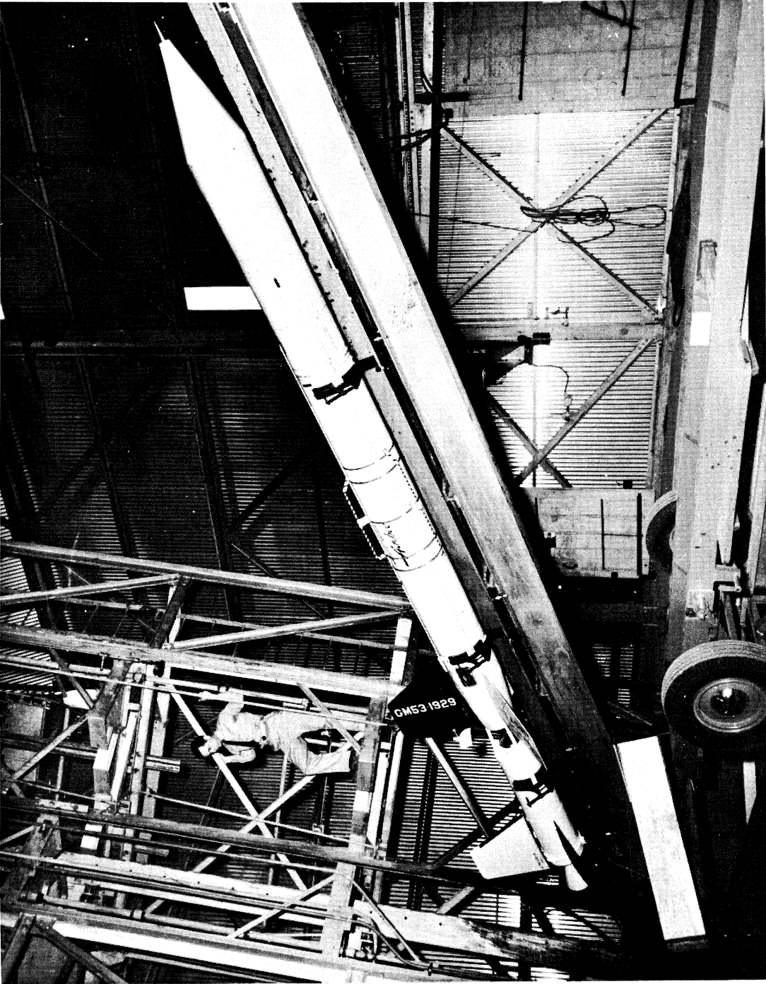
Fig. 2. Aerobee SM1:01 being raised up into launching tower.
