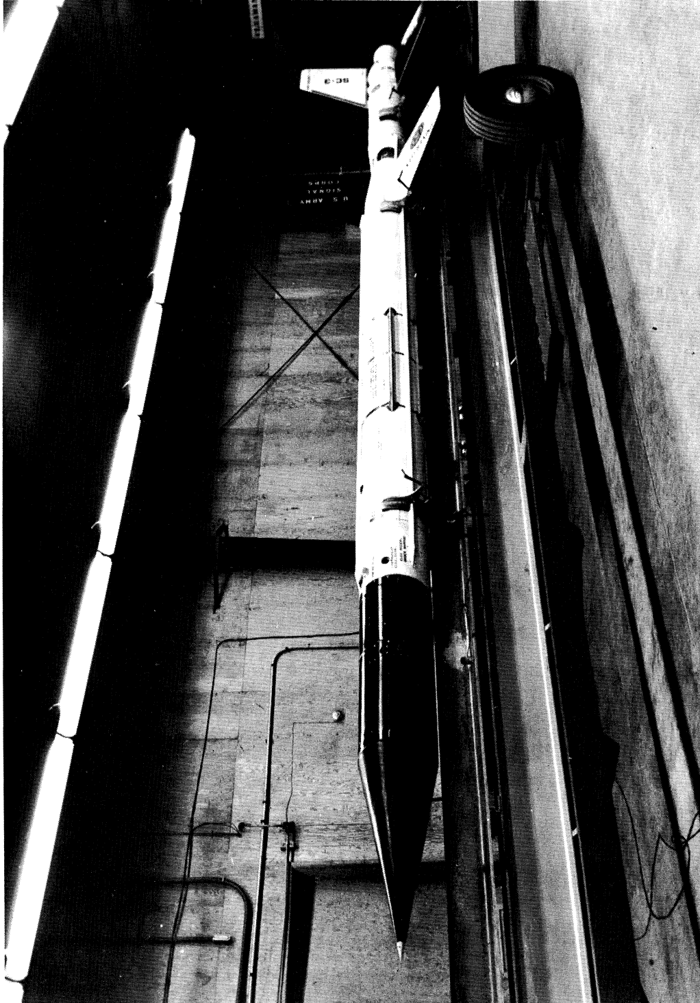
Fig. 1. SM2:06 ready for installation in the launching tower.
