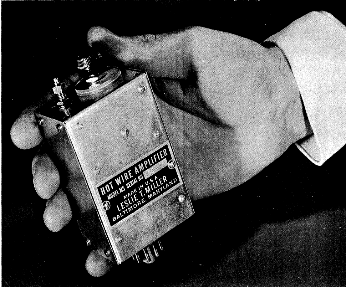
Figure 2-5. The model M-5 hot wire amplifier unit.
