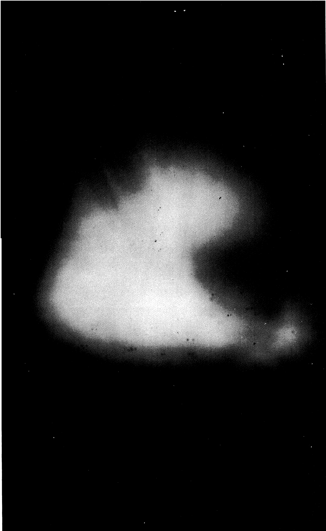
Fig. 10. Photograph of Burning Drops with Axis of Camera Horizontal (Plane of Picture Vertical) - Heated Air Supply.
