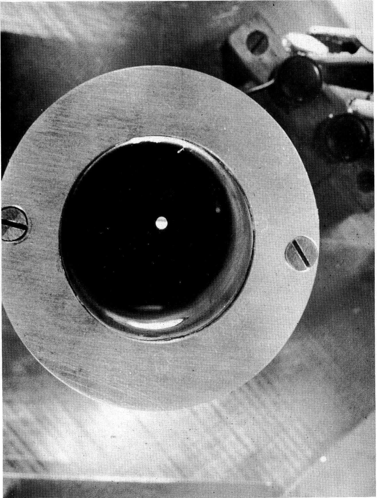
Fig. 25. Cork Ball Shown Suspended in Ultrasonic Tube. (Ball diameter - 0.1 in.)
