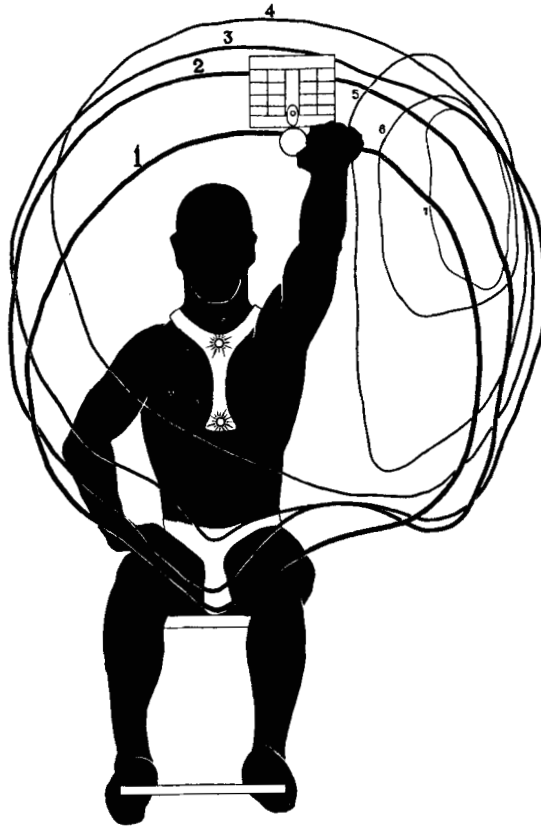
Fig. 3 Seven contour outlines show the range of movement of the prone hand over a series of frontal planes spaced at 6-inch intervals. The relative position of the seat and subject are shown also; the lights attached to the yoke over the sternum indicated whether or not trunk movement contributed to hand range.
