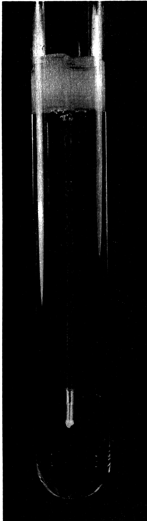
Fig. 1. Stainless Steel Cylinder Dissolving in Sulfuric Acid. Distance between Polyethylene Holder at Top and Polyethylene Cap at Bottom is Five Inches.
