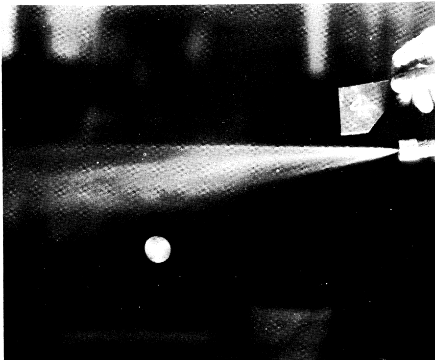
Fig. 4. Orifice nozzle, 128°F - 1.8% flashing.
