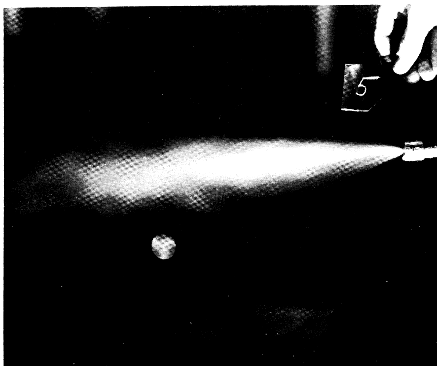
Fig. 5. Orifice nozzle, 256°F - 4.5% flashing.
