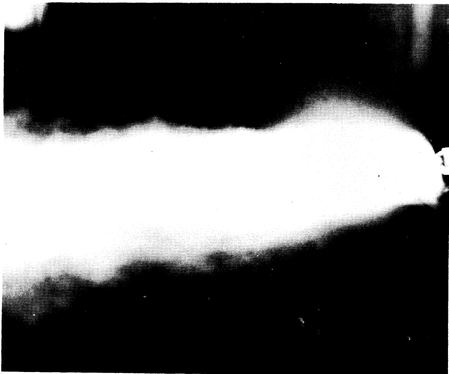
Fig. 13. Swirl nozzle, 324°F - 11.7% flashing.
