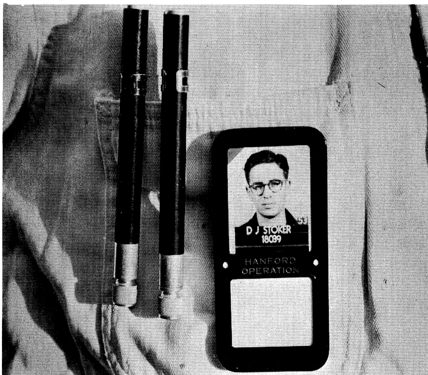
Figure 1.4 Pencils and badges worn to obtain records of radiation exposure (Courtesy of General Electric Co.)
