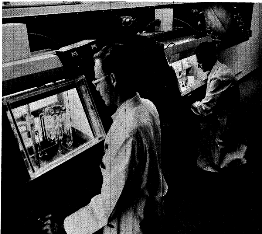
Figure 2.10 On the left, shielded-box assembly with ball-socket manipulators. On the right, standard gloved-box unit
