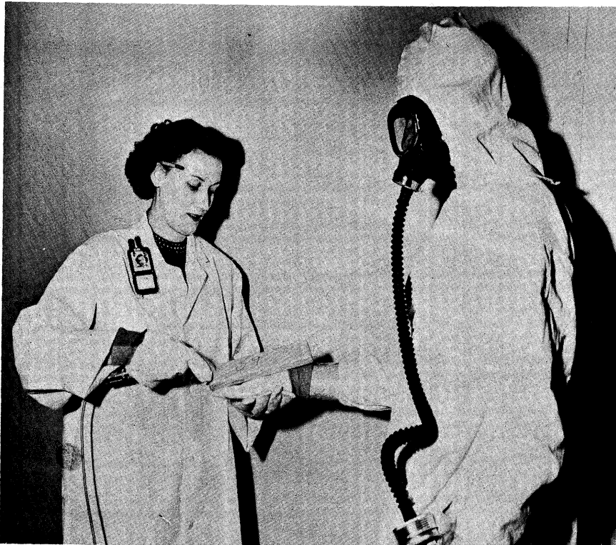
Figure 2.21 Worker with special suit for protection in radiocontaminated areas being checked for contamination. (Courtesy General Electric Co.)
