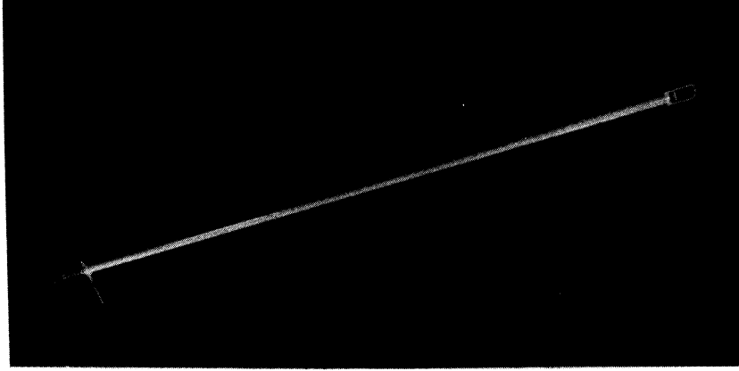
Fig. 22. Special Tool for Attaching and Removing Clips from Joints Located at Right Angle of the Access Chute to 10 kc Gamma Source.
