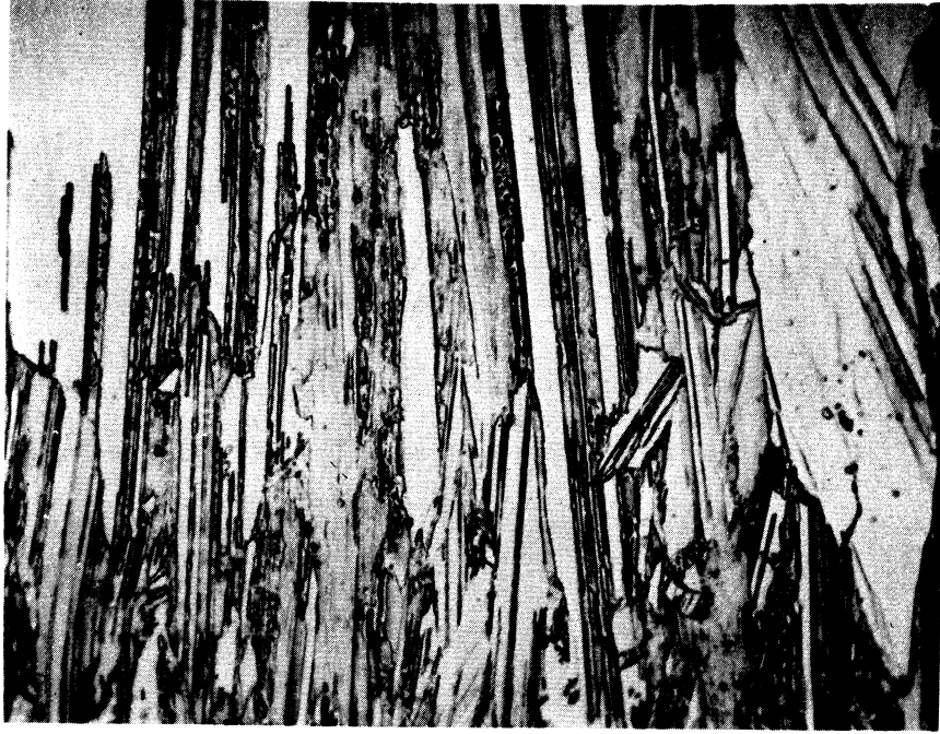
Fig. 30. Microstructure of "0.010 in." copper, \text{NH}_4\text{OH} , \text{H}_2\text{O}_2 etch, magnification 500x.
