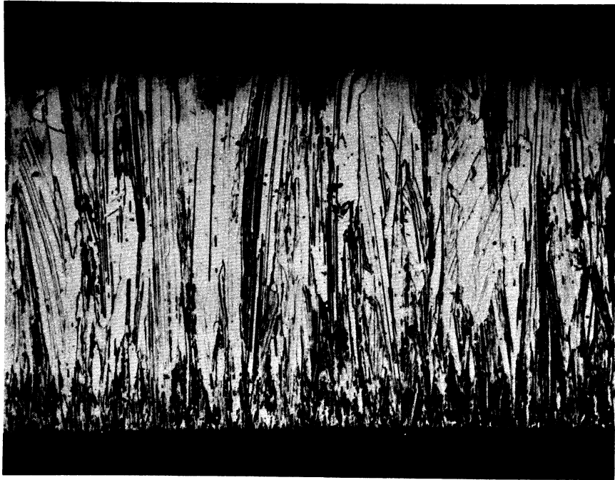
Fig. 31. Microstructure of "0.020 in." copper, \text{NH}_4\text{OH} , \text{H}_2\text{O}_2 etch, magnification 100x.
