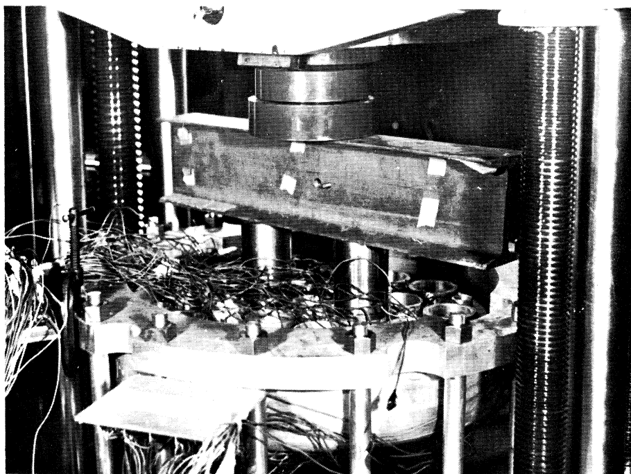
Fig. 13. General test arrangement for axial loading of aluminum shell.
