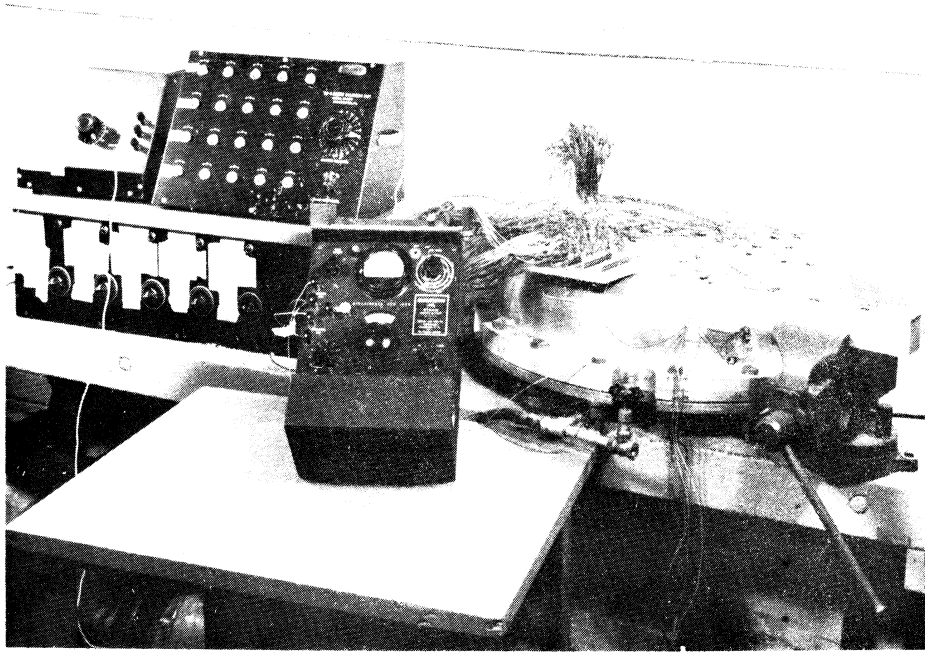
Fig. 1. Shell, switch boxes, and bridge in place for pressure test.
