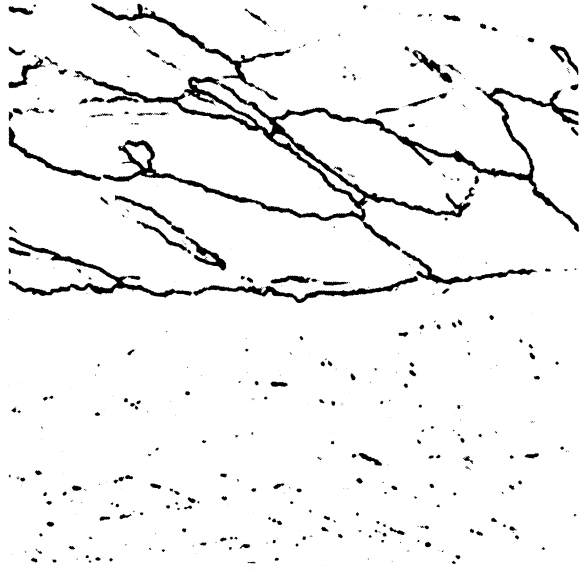
(c) Heated 45 Minutes at 1800°F, Rolled 59.3 Percent in 6 Passes, Air Cooled.
