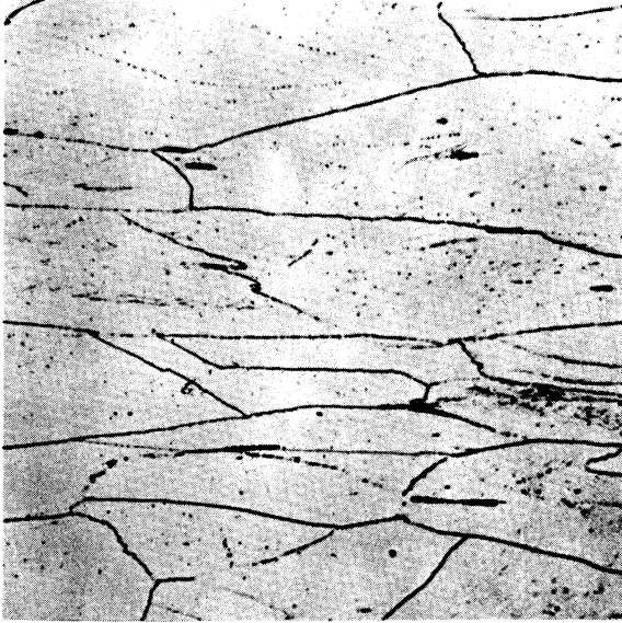
(c) Heated 45 Minutes at 1400°F, Rolled 58.7 Percent in 6 Passes, Air Cooled.
