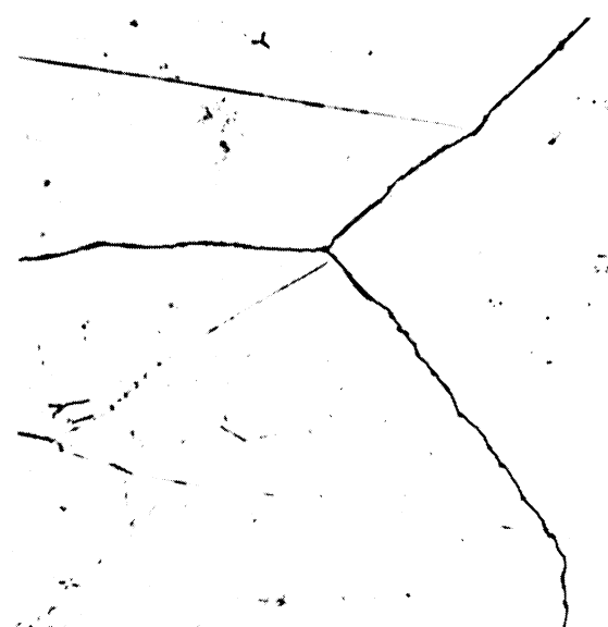
(b) Heated 45 Minutes at 1400°F, Rolled 19.5 Percent in 3 Passes, Air Cooled.
