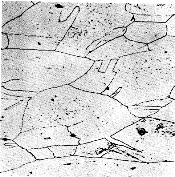
(d) Heated 45 Minutes at 1400°F, Rolled 36.1 Percent in 2 Passes, Air Cooled.
