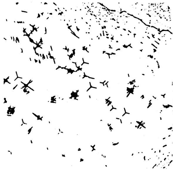
(a) Base Condition. (As Received + 20 Percent Cold Work + 1 Hour at 1600°F, Air Cooled.)
