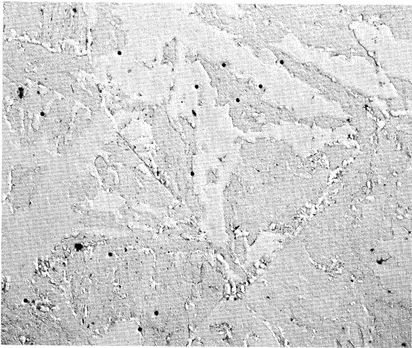
(b) 1 Hr. 2200°F, AC to 2100°F, Rolled 50% Red. in 2 Passes, AC + Tempered 6 Hrs. at 1250°F; BHN-326; G.S. -7.5.
