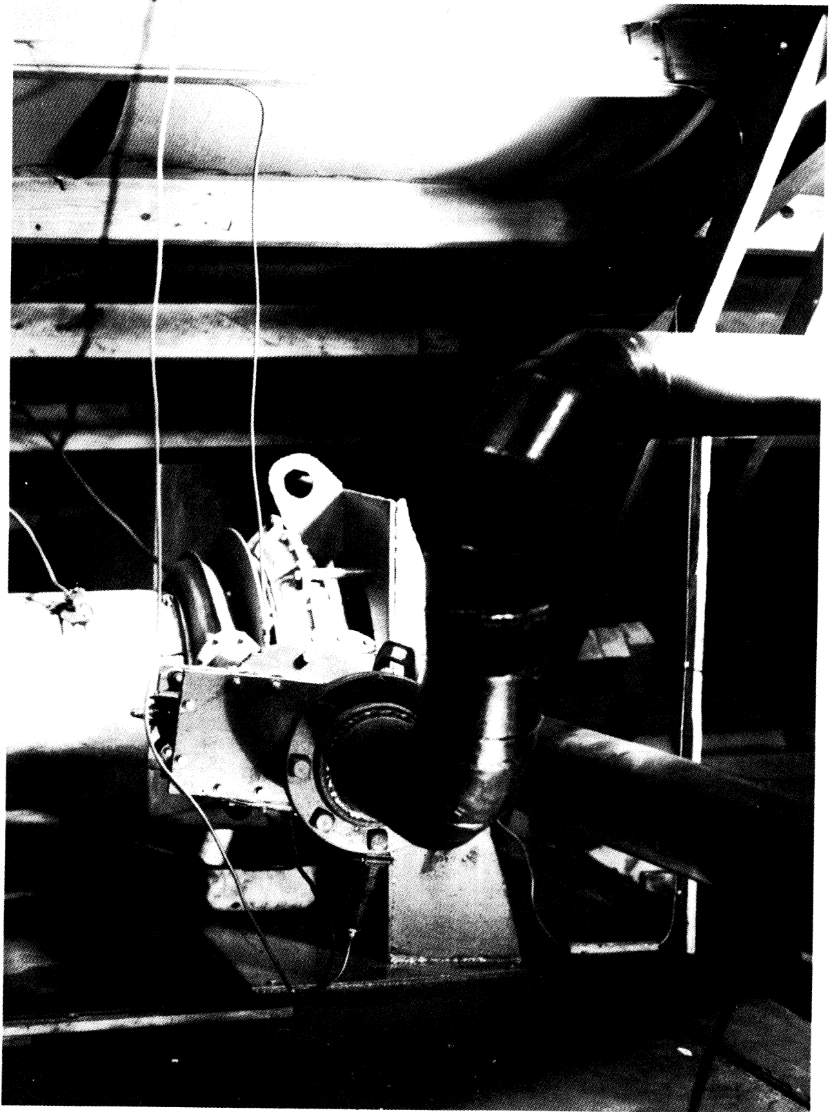
Fig. 10 - Photograph of a B-22 Type Turbo-Supercharger Used as an Expansion Turbine
