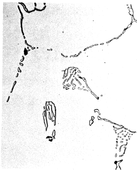
(d) One minute at 2480°F, furnace cooled to 2350°F, held 10 minutes at 2350°F, A.C. Very coarse structure of CbC and austenite.
