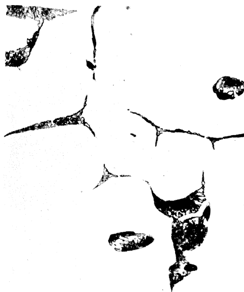
(b) One minute at 2480°F, A.C. The dark grey structure is rich in Fe_2Cb .
