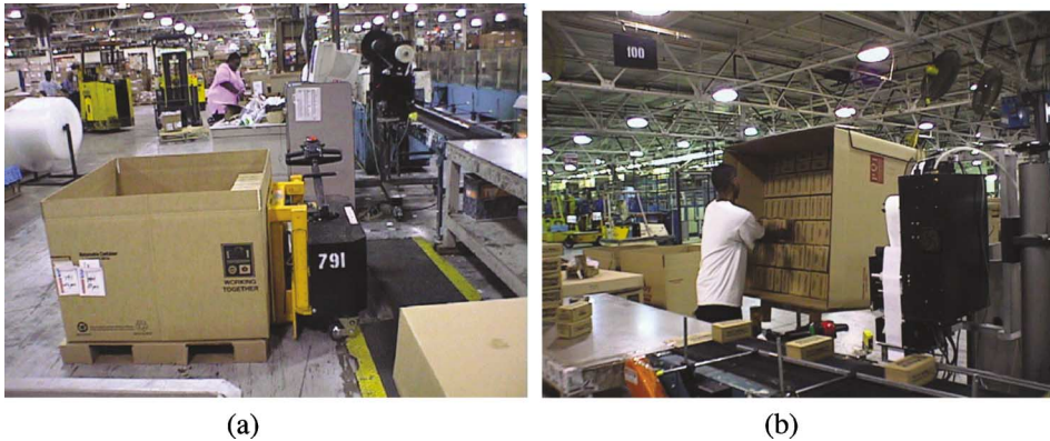
Fig. 8. Lift/tilt pallet jack — a combination pallet jack and lift/tilt device. Panel 2(a) shows the lift/tilt pallet jack positioned under a triwall on the floor. Panel 2(b) shows the lift/tilt pallet jack with a raised triwall.
