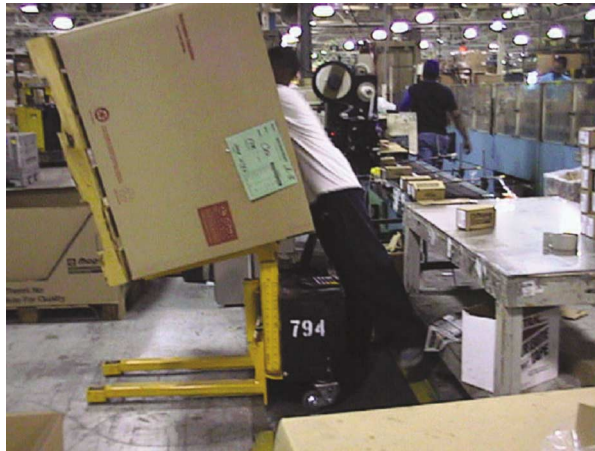
Fig. 9. Lift/tilt pallet jack in intermediate position.
