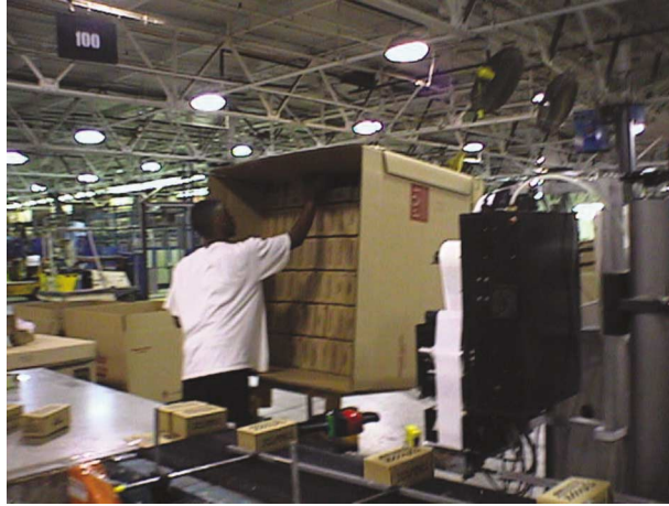
Fig. 10. Workers must elevate their shoulders when working with the lift/tilt pallet jack in the fully elevated position.
