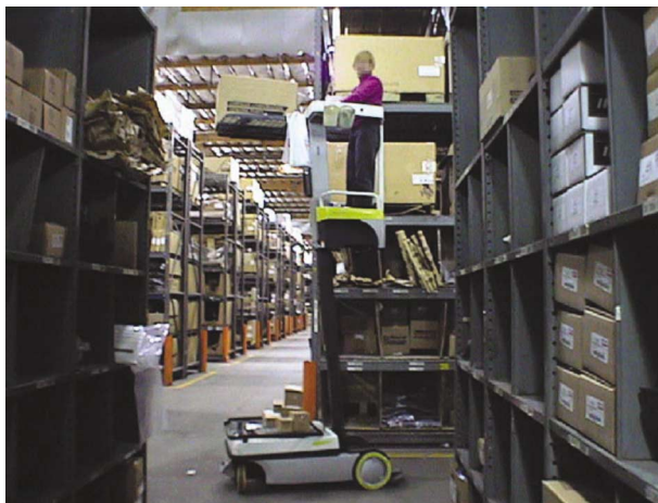
Fig. 4. Elevated vertical position of the self-elevating vehicle (used for stocking and picking).
