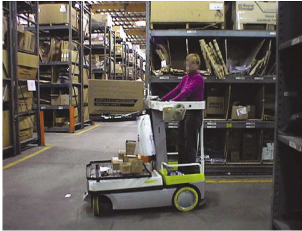
Fig. 3. Lowest vertical position of the self-elevating vehicle (used for horizontal movement).
