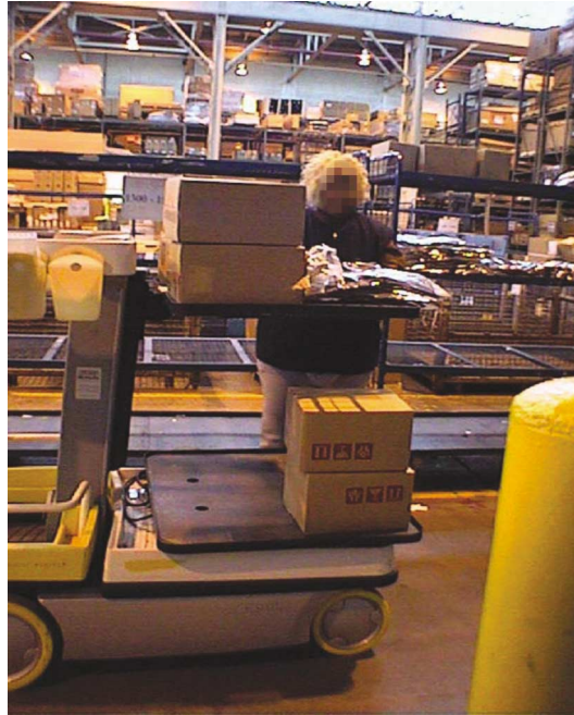
Fig. 6. Boxes stacked higher than shoulder height on the self-elevating vehicle which would lead to shoulder elevation.
