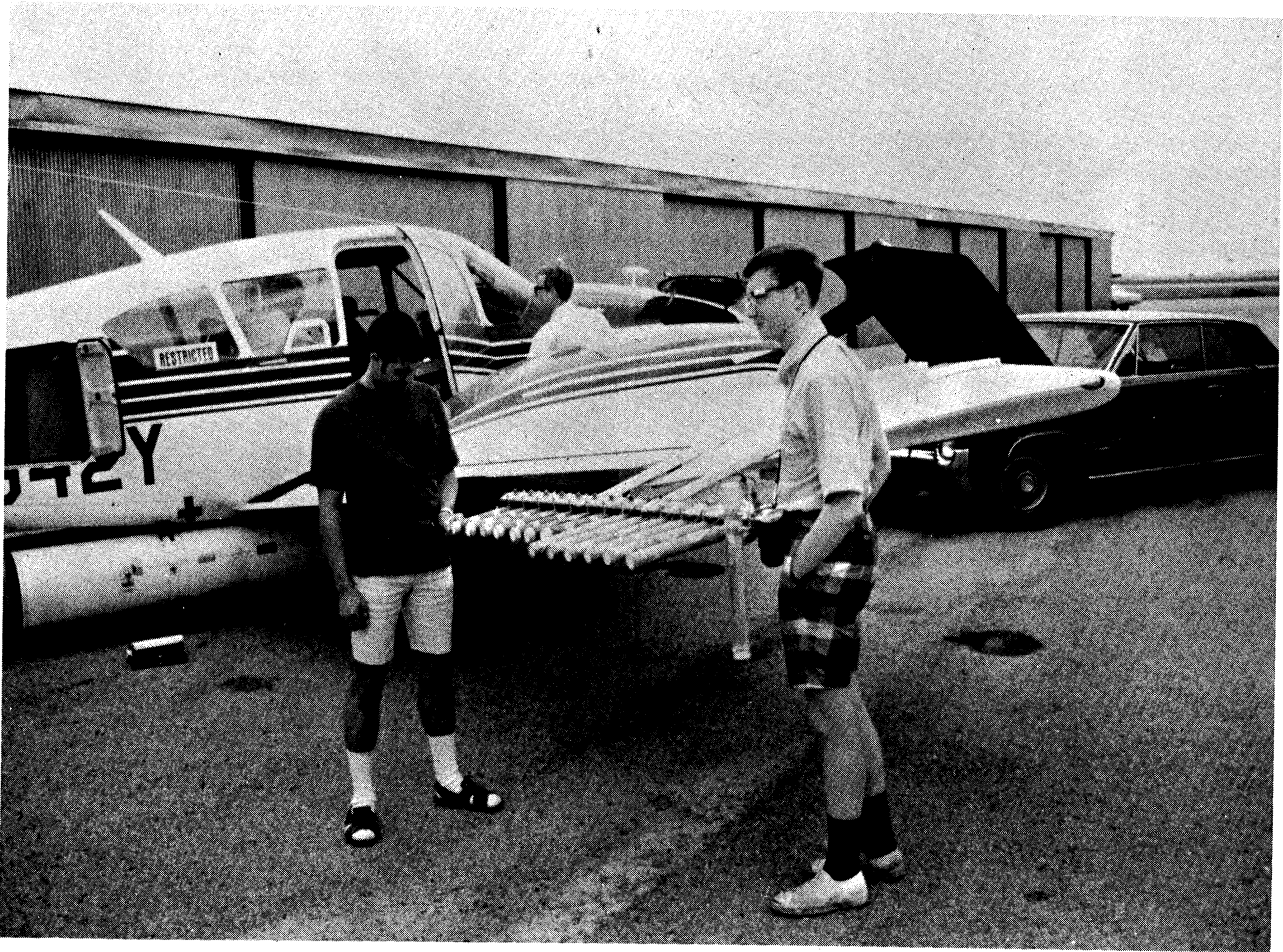
Figure 35. The Piper Aztec airplane of Weather Service, Inc., used to place indium tracer; flares in place under inspection by Messrs. James Fairbent, left, and David Curtin, right, of The University of Michigan research team.
