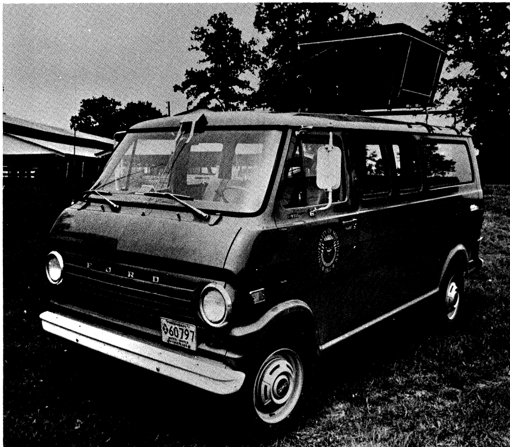
Figure 13. One of two University of Michigan Mobile units with rooftop rain collector. (WSI photograph)
