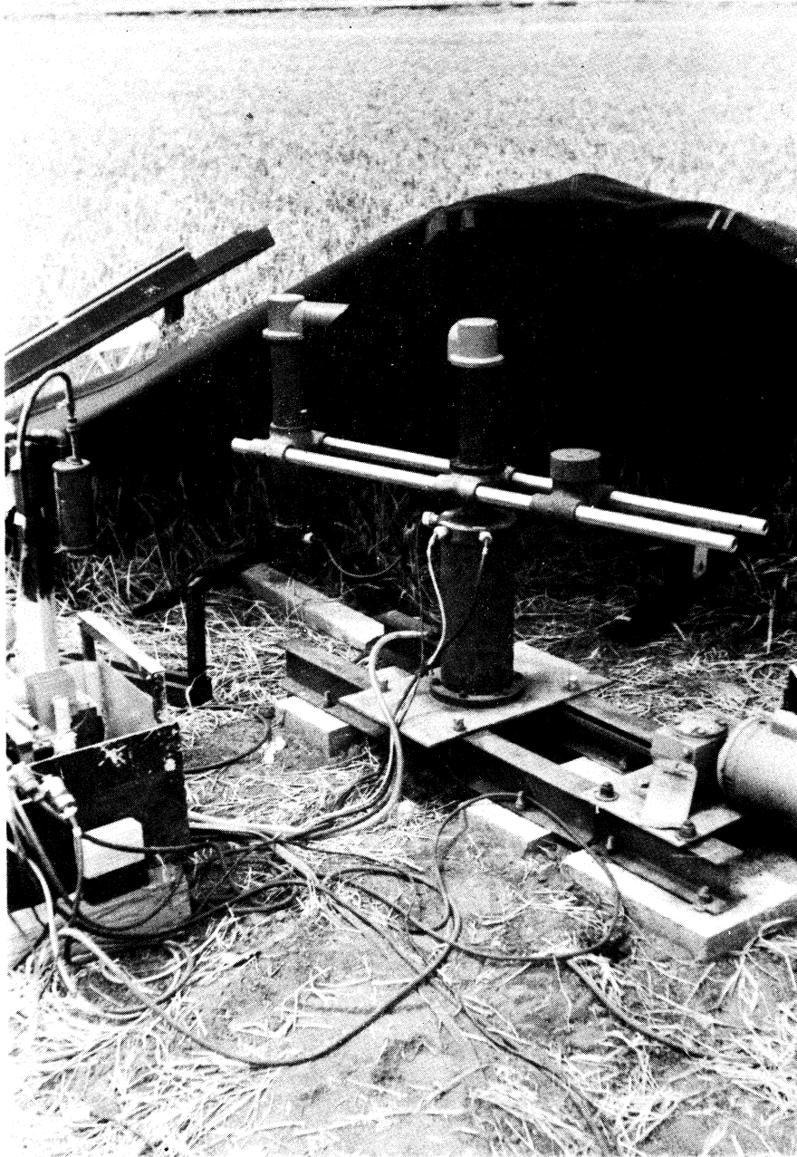
Figure 8. The raindrop-size spectrometer and associated equipment with the tent folded back.
