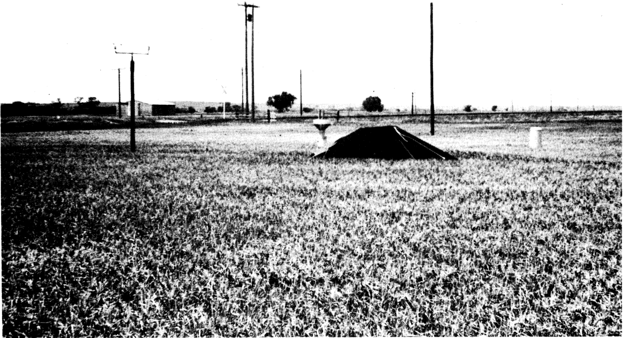
Figure 4. View looking SW. The black tent houses the raindrop spectrometer. The tipping bucket (right) and weighing (center) raingauges, and the anemometer-wind vane assembly (left) are shown.
