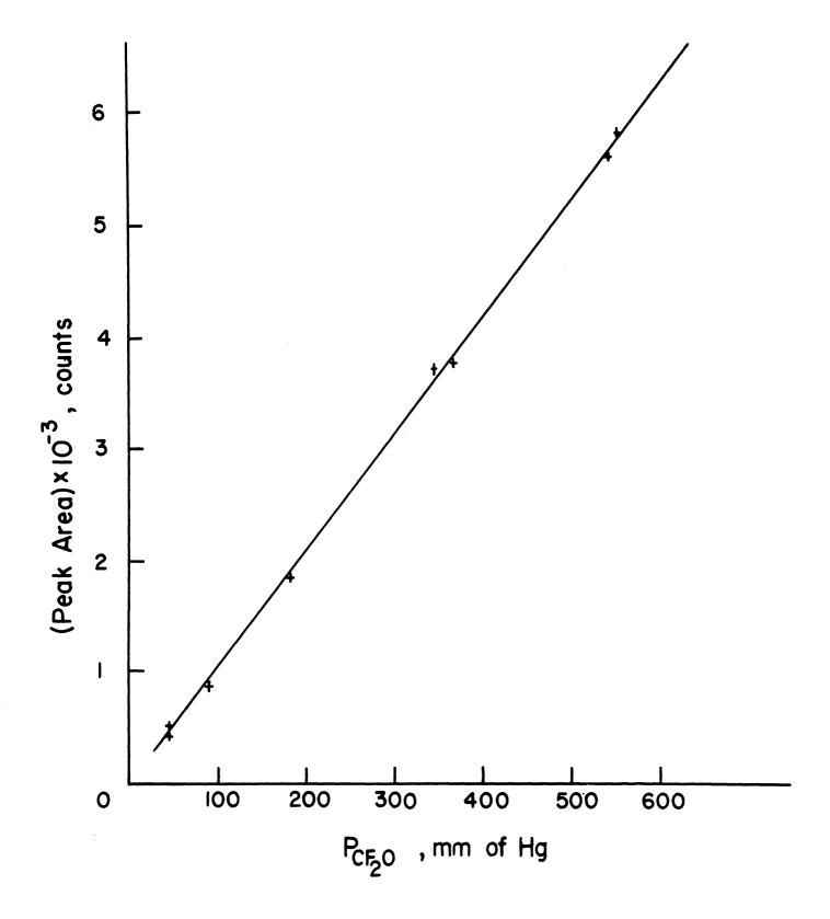
FIG.2 CF<sub>2</sub>O PEAK AREA AS A FUNCTION OF SAMPLE PRESSURE
