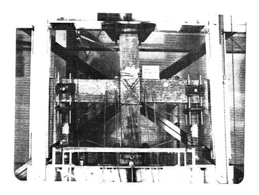
Fig. 2.9 An X-Series Specimen in the Testing Frame
