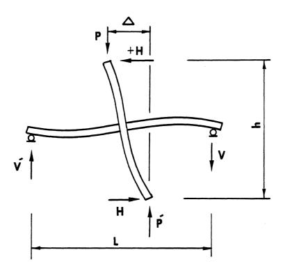
Fig. 2.2 Deformed Shape of Beam-Column Subassemblage
