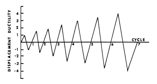
Fig. 2.11 Typical Loading Routine
