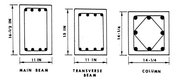
Fig. 2.5 Beam, Slab and Column Cross Sections
