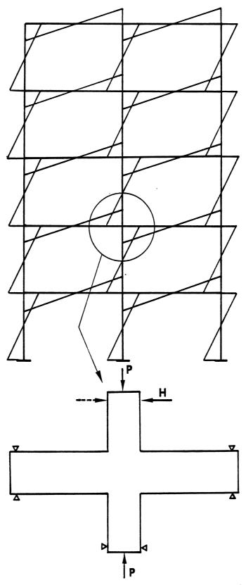
Fig. 2.1 Test Subassembly of Beam to Column Connection
