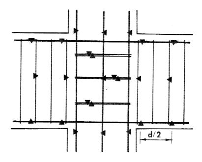
Fig. 2.10 Typical Strain Gage Location in an X-Series Specimen
