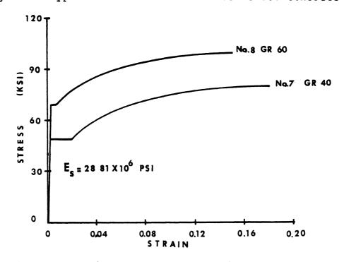
Fig. 2.7 Typical Stress vs. Strain Curve for Steel
