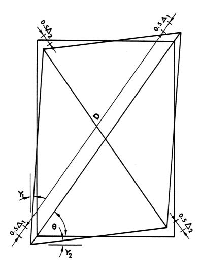
Fig. 3.4 Joint Shear Deformation Model
