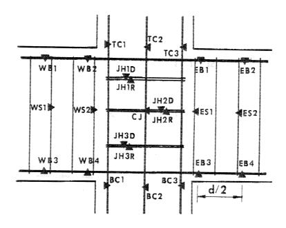
Fig. E.1 Gage Locations in X-series Specimens
