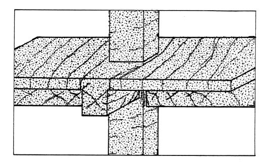
Fig. 3.2 Typical Cracking Pattern in a S-Series Specimen
