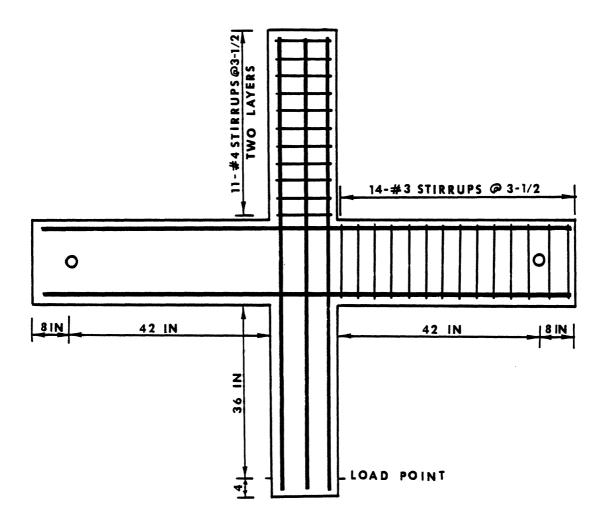
Fig. A.1 Typical Beam and Column Shear Reinforcement
