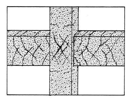
Fig. 3.1 Typical Cracking Pattern in an X-Series Specimen
