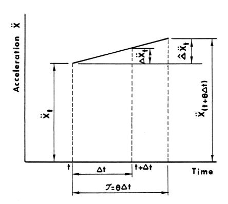
Fig. 5.7 Linear Acceleraion over Extended Time Period
