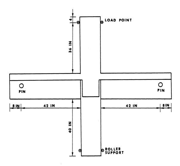
Fig. 2.4 Overall Dimensions of a Specimen
