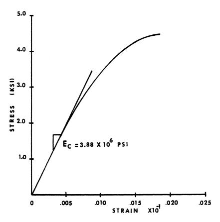
Fig. 2.6 Typical Stress vs. Strain Curve for Concrete
