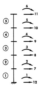
Fig. 5.5 Numbering Scheme for Global Degrees of Freedom
