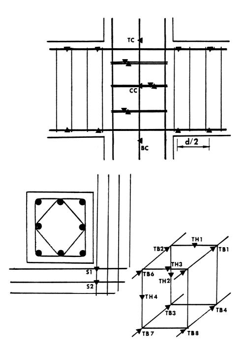
Fig. E.2 Gage Locations in S-series Specimens
