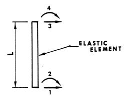
Fig. 5.4 Nodal Degrees of Freedom of an Element
