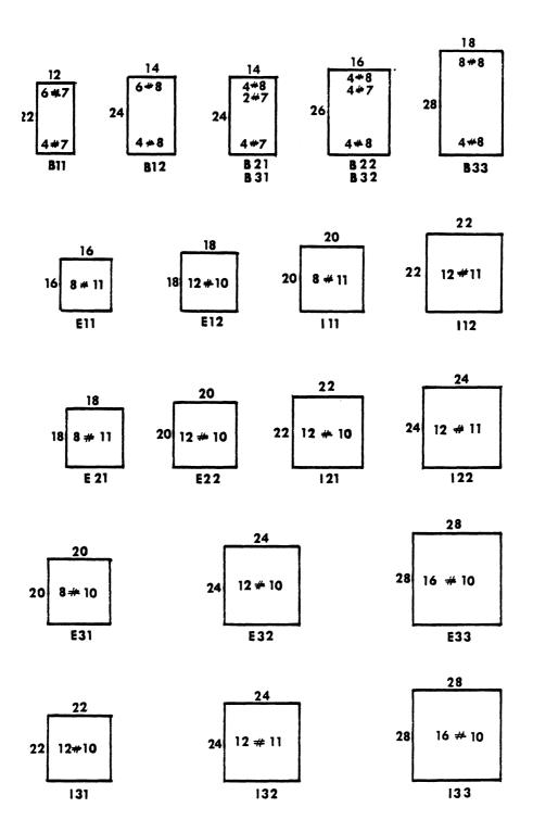
Fig. 6.2 Cross Sectional Details of Frame Members
