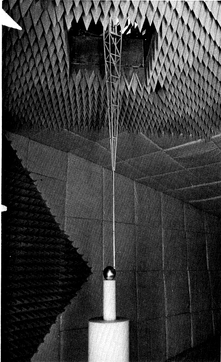
FIG. 4-23: ANTENNA NO. 223 WITH MAGNETIC PROBE ABOVE THE SURFACE; SHOWN IN ANECHOIC CHAMBER
