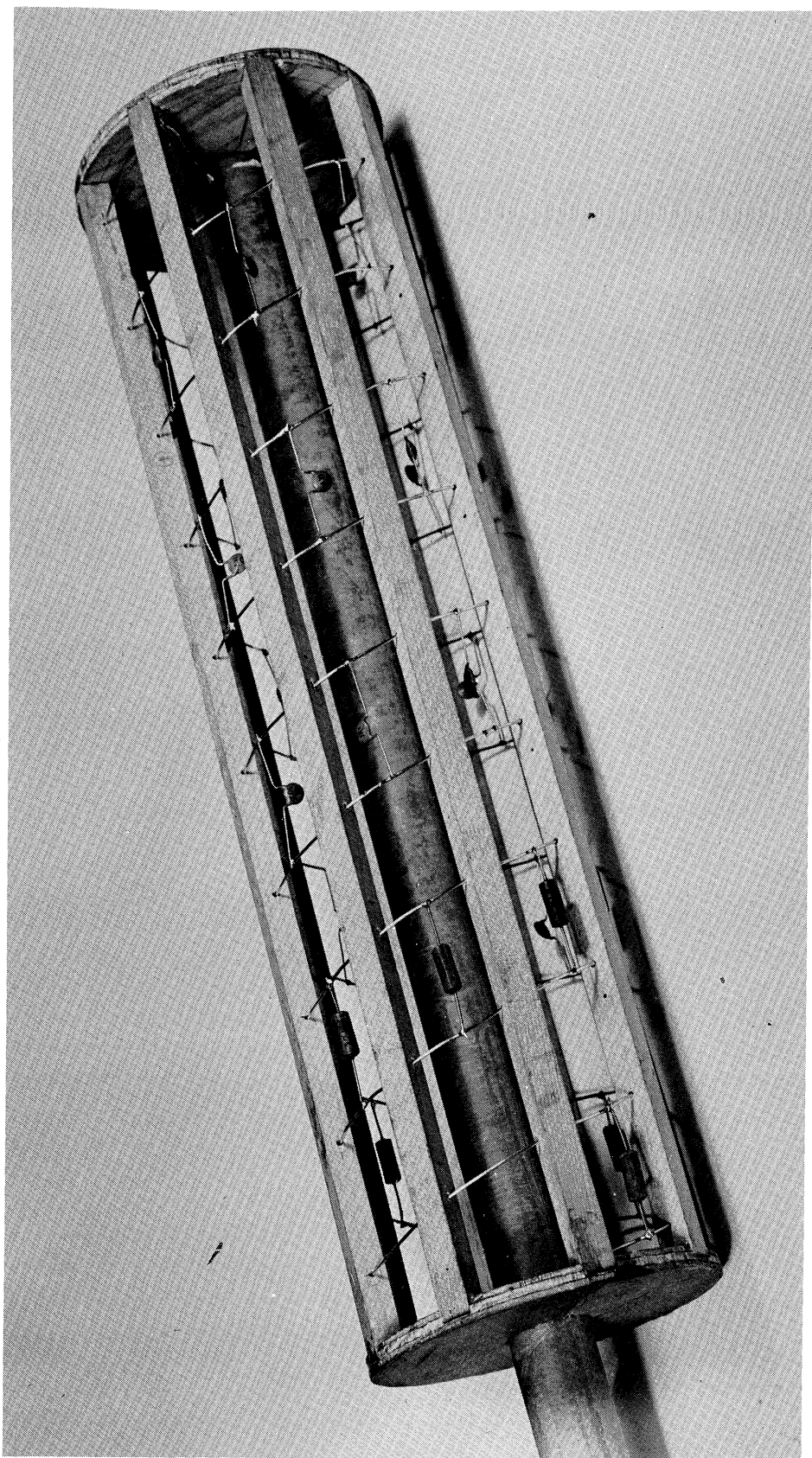
FIG. 3-14: PHOTOGRAPH OF ANTENNA 224 WITH 12 pf CAPACITORS IN TYPE I LOADING.
