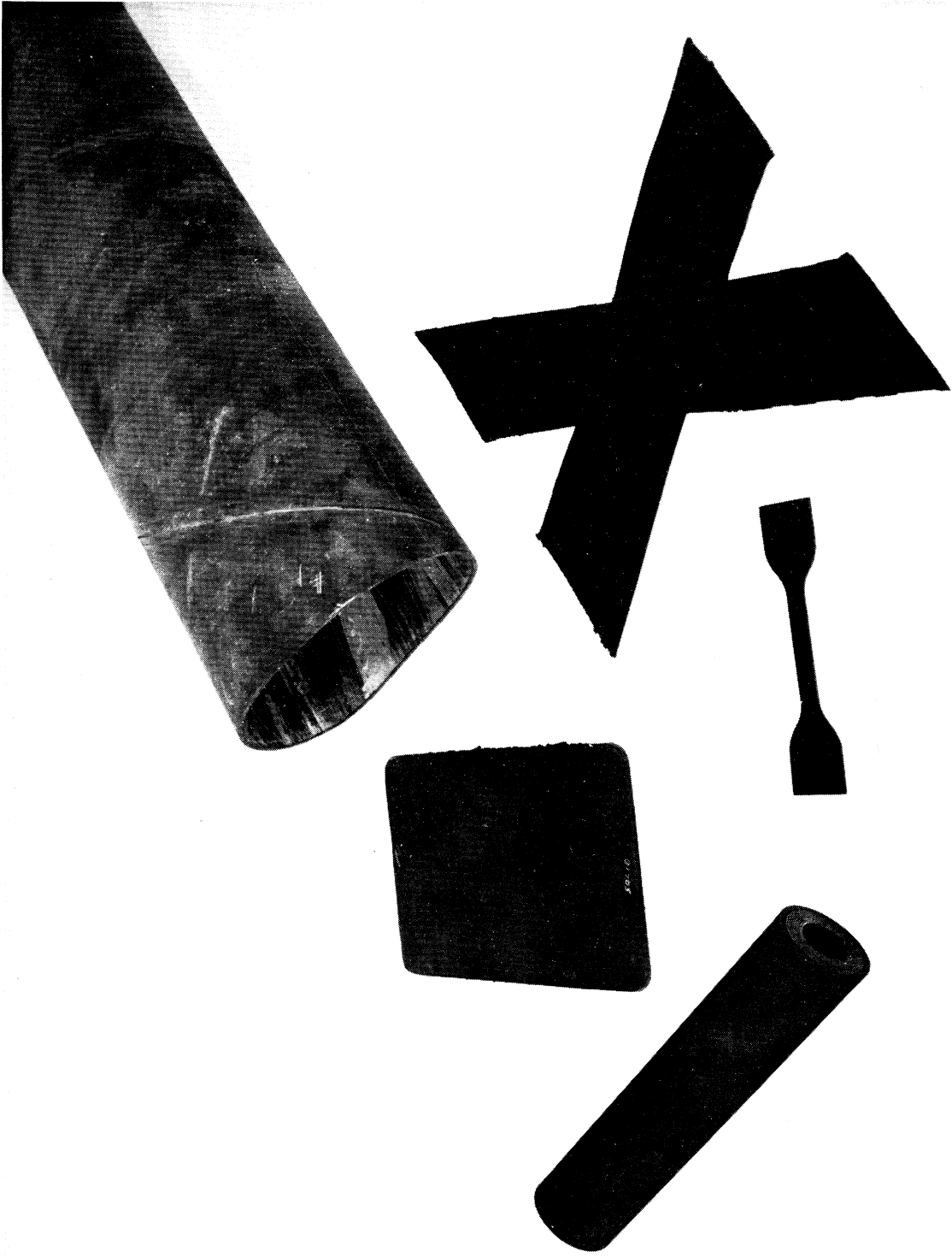
Fig. 3. Typical specimens used in determining the elastic properties of carcass structures.
