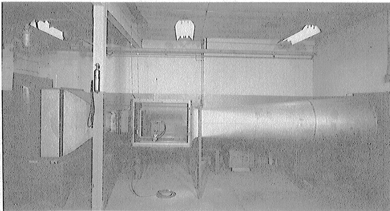
Fig. 1. Overall View of Wind Tunnel and Test Section
