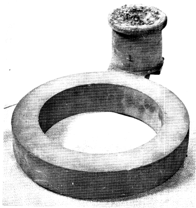
Fig. 11b. Shell-cast rear follower, Part No. 7359510. Reduced to 1/8 size.
