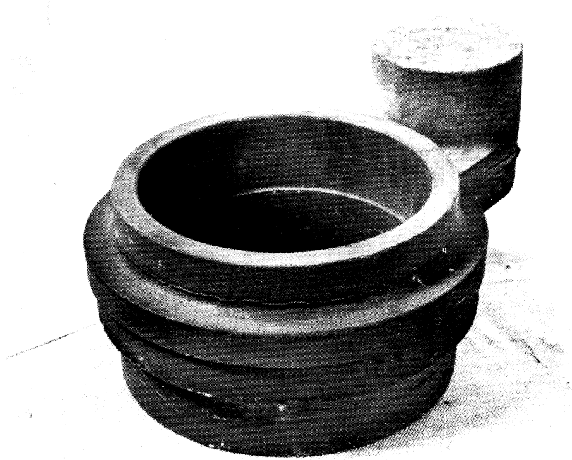
Fig. 11a. Shell-cast front follower, Part No. 7360356. Reduced to 1/8 size.
