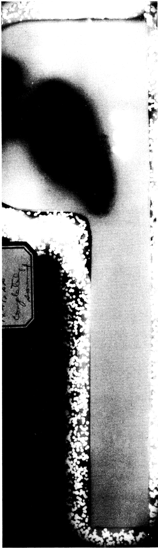
Fig. 6. Radiographs showing effect of feeding distance on centerline shrinkage
