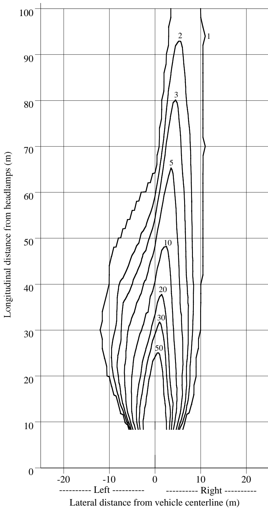
Figure 8. Isoillumination diagram (in vertical lux) at the road surface from a pair of lamps having the median (50th percentile) luminous intensities for the sales-weighted sample representing the low-beam headlamps on current passenger vehicles in Europe. (Test voltage: 12.8 V. Lamp mounting height: 0.62 m. Lamp separation: 1.12 m.)
