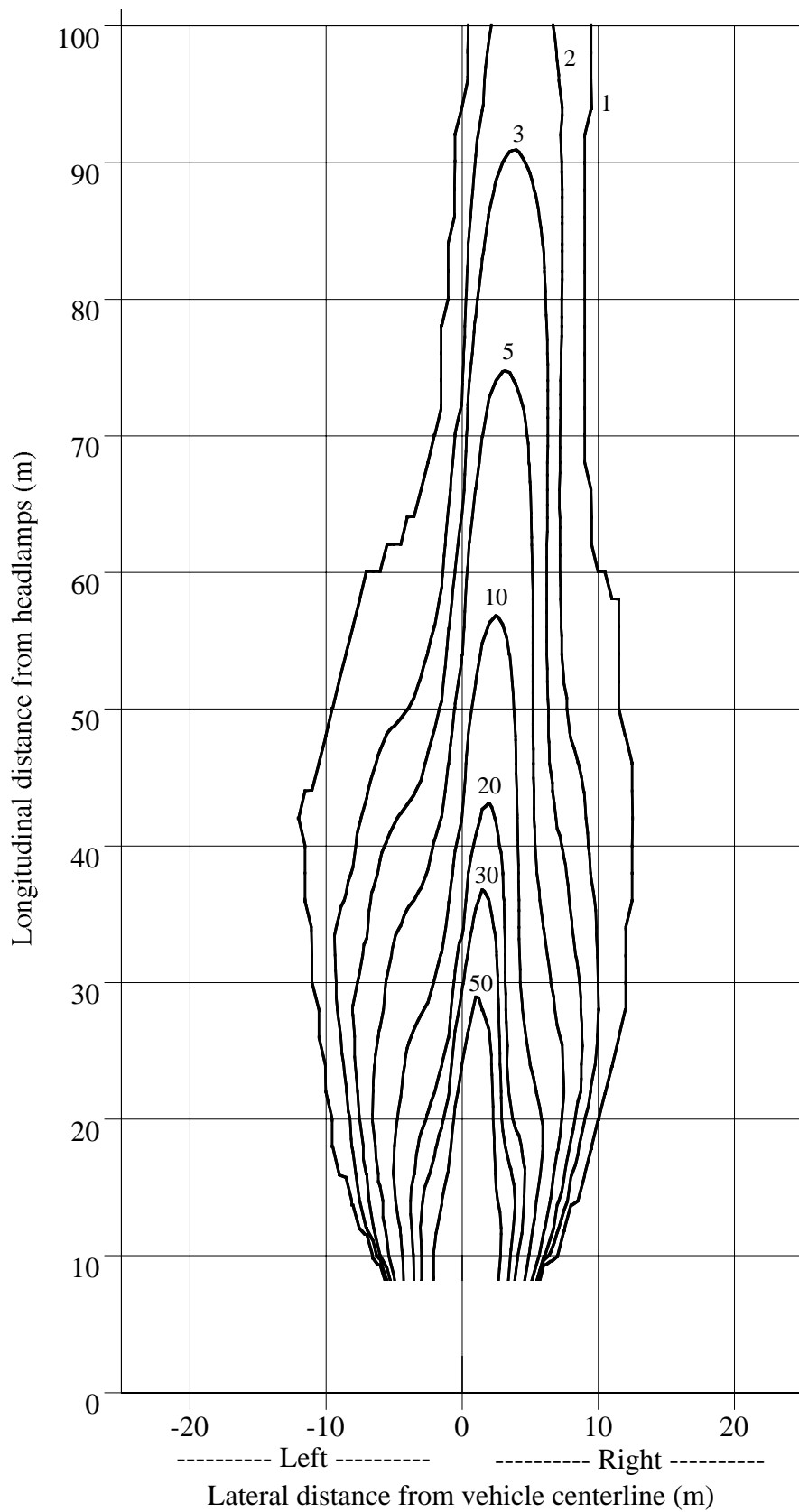
Figure 7. Isoillumination diagram (in vertical lux) at the road surface from a pair of lamps having the median (50th percentile) luminous intensities for the sales-weighted sample representing the low-beam headlamps on current passenger vehicles in the U.S. (Test voltage: 12.8 V. Lamp mounting height: 0.62 m. Lamp separation: 1.12 m.)
