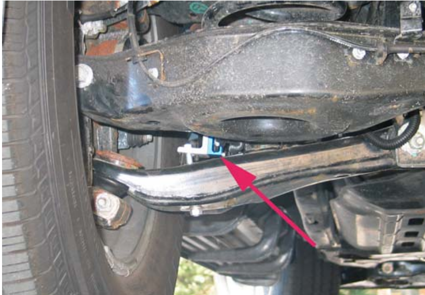
Figure 2.6. Left-rear accelerometer installation (unsprung-mass data)
