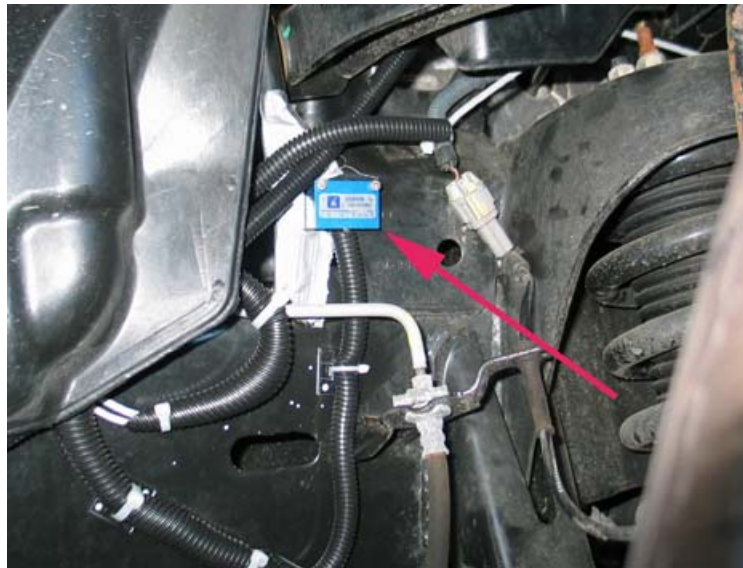
Figure 2.5. Right-front accelerometer installation (sprung-mass data)
