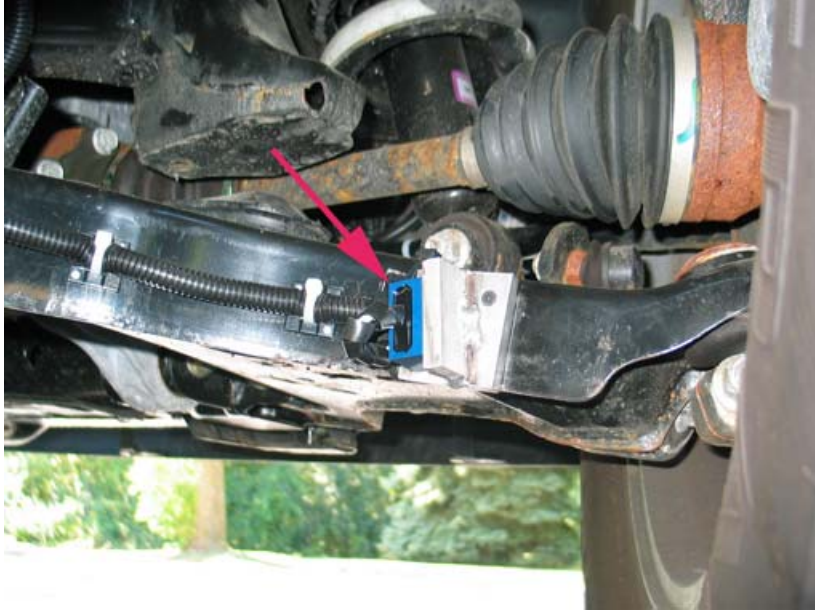
Figure 2.4. Right-front accelerometer installation (unsprung-mass data)
