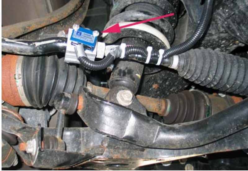
Figure 2.2. Accelerometer installation at the right-side of the steering tie rod
