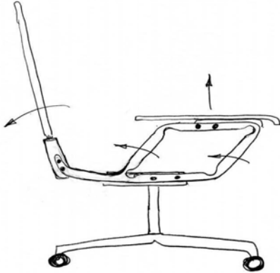
Figure 10: Final Concept for Compliant Synchronized Reclined System
