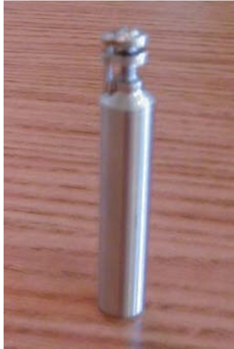
Figure L: Manufactured Cylindrical Jig Used in the Bending of the Stainless Steel Cooling Channel
