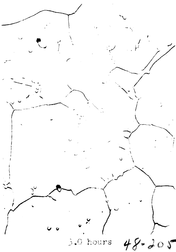
Cross section of bar X1000 Electrolytically etched in 10 percent chromic acid
