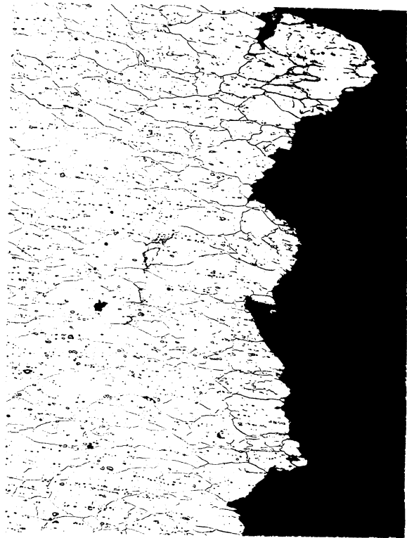
Aged 100 hours: failed in 0.05 hours under a stress of 80,000 psi 49-27
