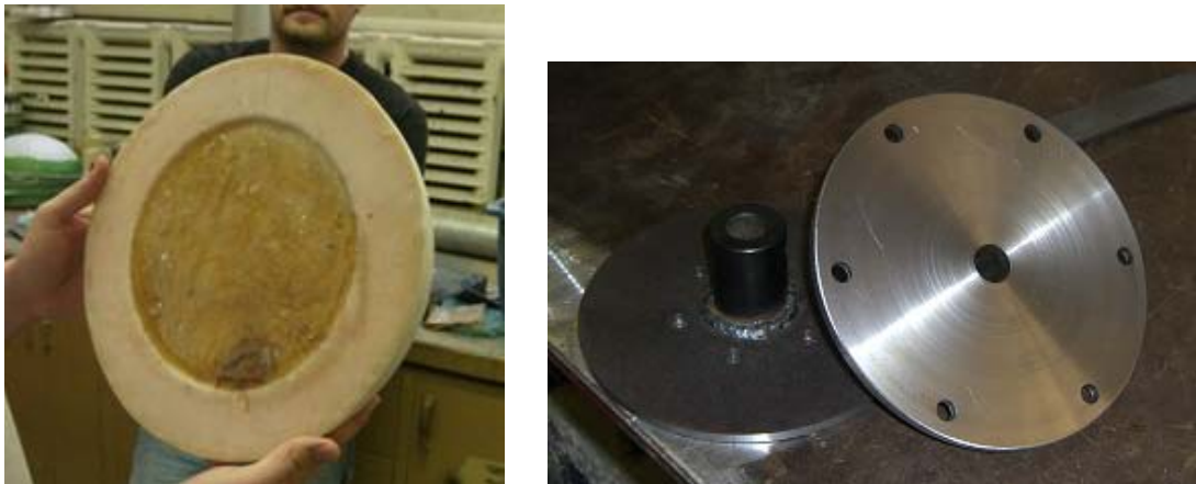
Figure 11: Blade to driveshaft coupler
