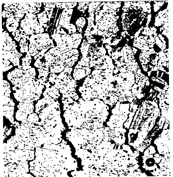
Figure 43 100x Spec. C1-15 Creep-Exposure 484 hours at 1800°F to 9.8% Deformation, Then Tensile Tested at Room Temperature
