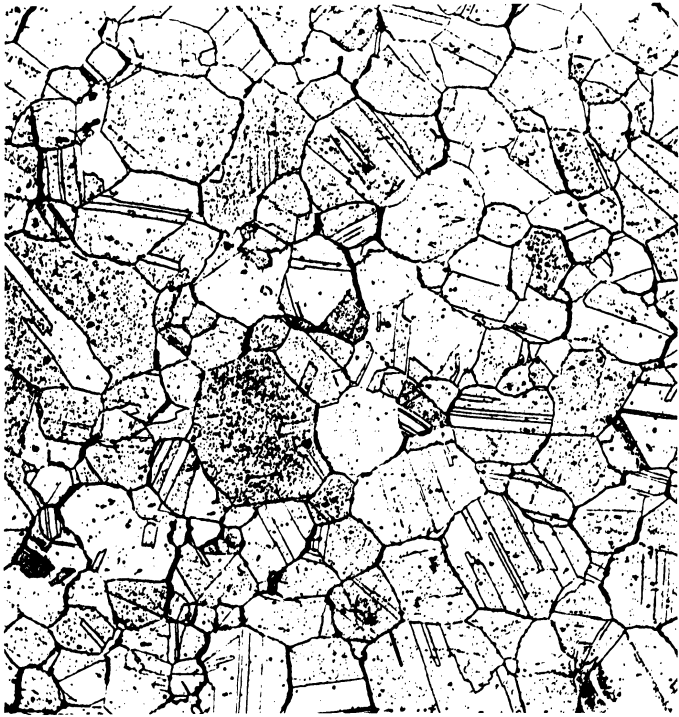
Figure 48 100x Spec. C2-61 Creep-Exposure 5 hours at 1600°F to 9.2% Deformation, NOT Tensile Tested
