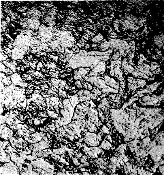
Figure 68 500x TZM As-Received (Transverse Section) (Rolled and Stress-Relieved)
