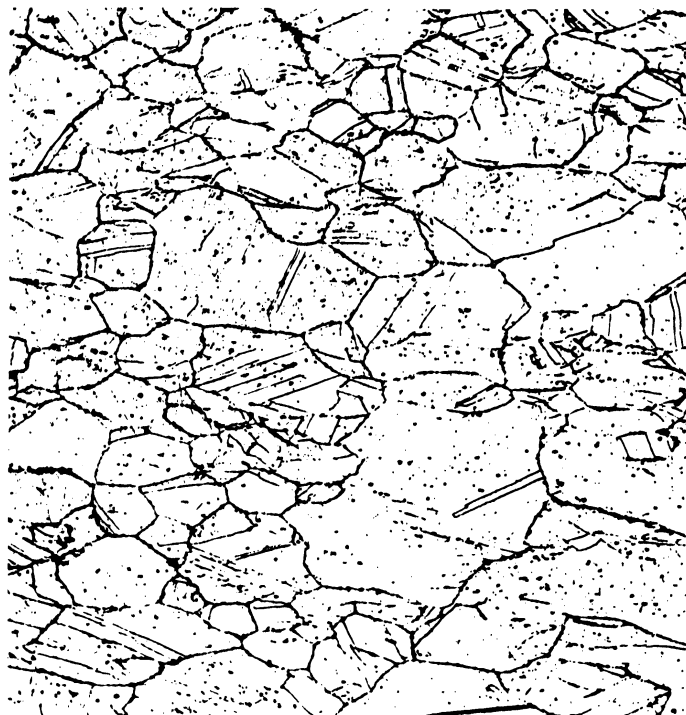
Figure 53 Spec. C2-60 Creep-Exposure 100 hours at 1800°F to 0.6% Deformation, Then Tensile Tested at Room Temperature
