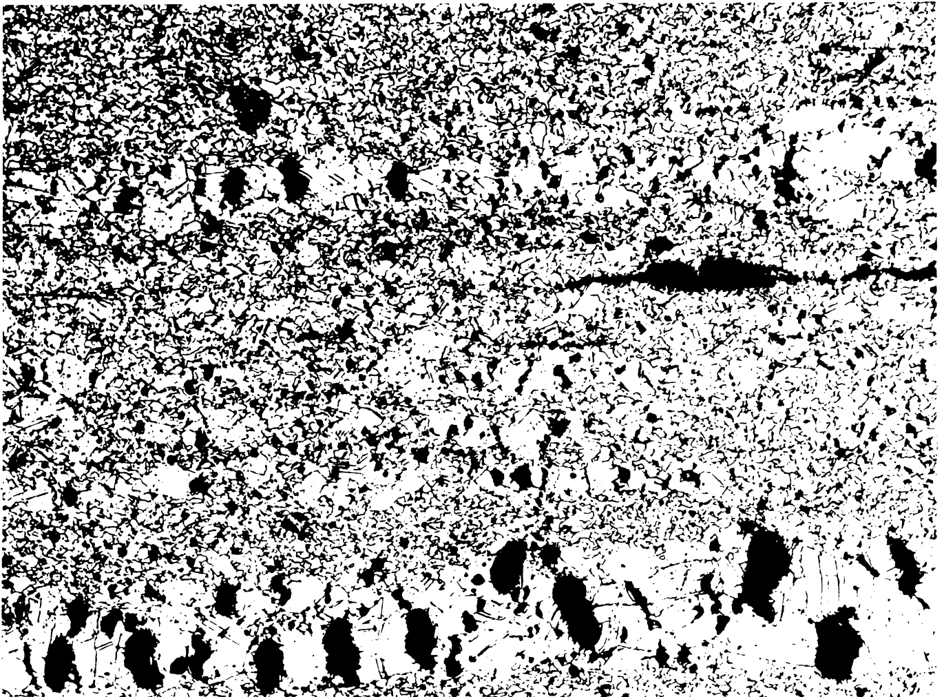
Figure 38 Approx. 120x Spec. C1-46 Creep-Exposure 100 hours at 1600°F to 10.5% Deformation, Then Tensile Tested at Room Temperature
