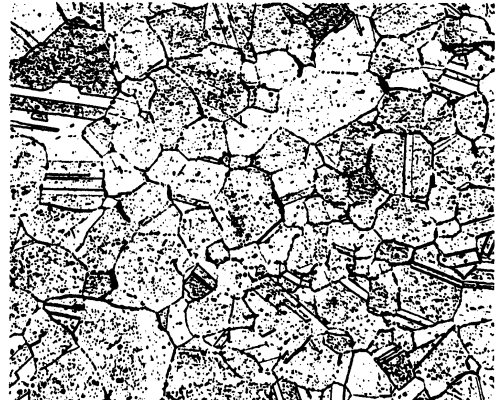
Figure 27 100x Spec. No. C2-5: 1600°F - 8000 psi. Failed at 4.7 hrs.
