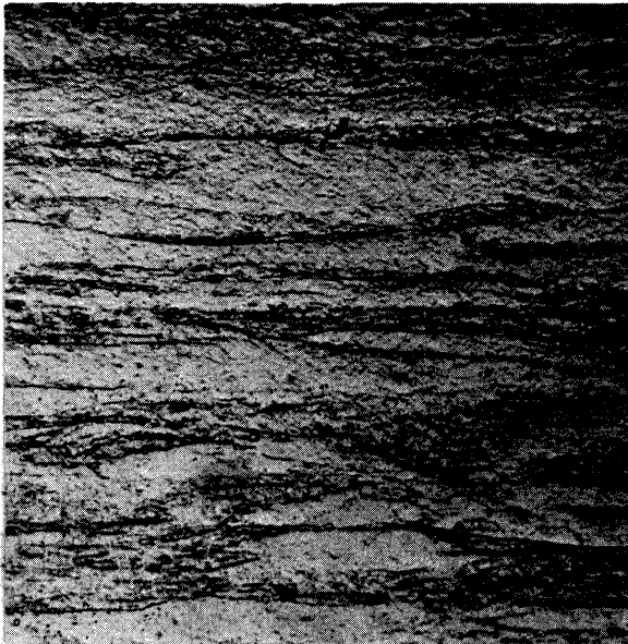
Figure 70 500x TZM Spec. M-4 Creep-Exposure 10 hours at 1800°F to 4.26 Percent Deformation, Then Tensile Tested at Room Temperature
