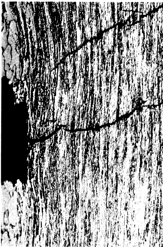
Figure 72 Fracture Area of Specimen M-3 After Creep-Exposure 10 Hours at 1800°F in Vacuum to 2.25-Percent Deformation And Then Tensile Tested at Room Temperature
