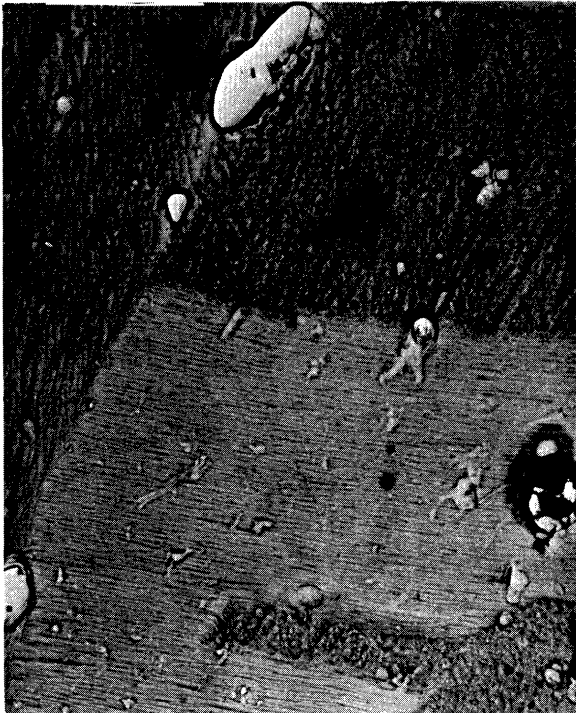
Figure 61 3500x Spec. C2-62 Creep-Exposure 50 hours at 1600°F to 3.8% Deformation
