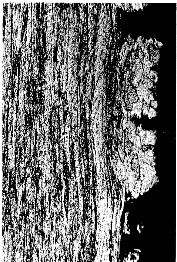
Figure 72 Fracture Area of Specimen M-3 After Creep-Exposure 10 Hours at 1800°F in Vacuum to 2.25-Percent Deformation And Then Tensile Tested at Room Temperature
