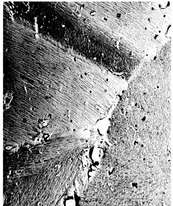
Figure 62 3500x Spec. C2-50 Creep-Exposure 5 hours at 1800°F to 4.8% Deformation
