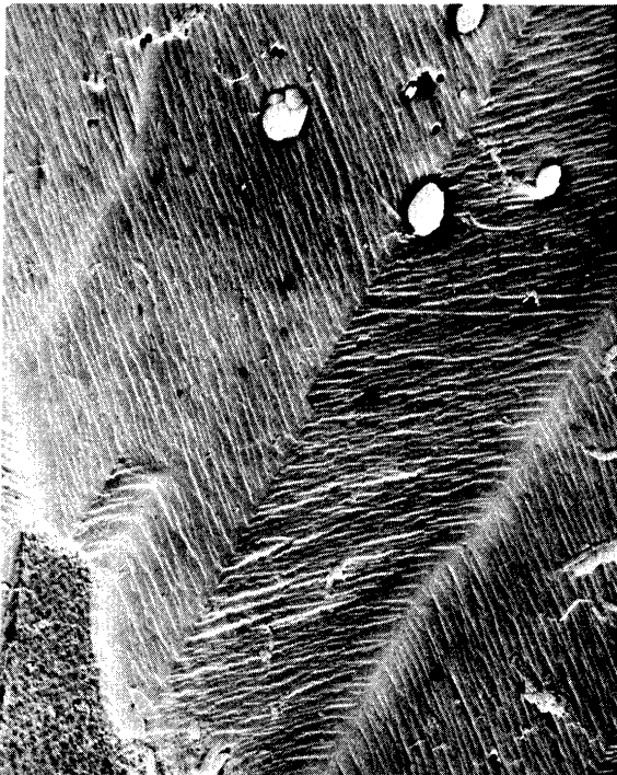
Figure 57 3500x Spec. C1-22 Creep-Exposure 5 hours at 1800°F to 2.5% Deformation
