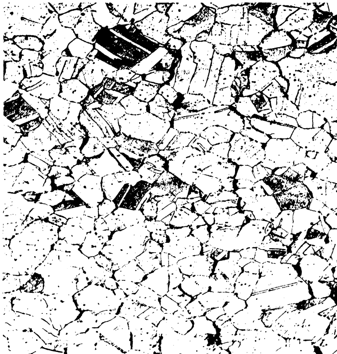
Figure 50 100x Spec. C2-44 Creep-Exposure 5 hours at 1600°F to 7.5% Deformation, Then Tensile Tested at Room Temperature
