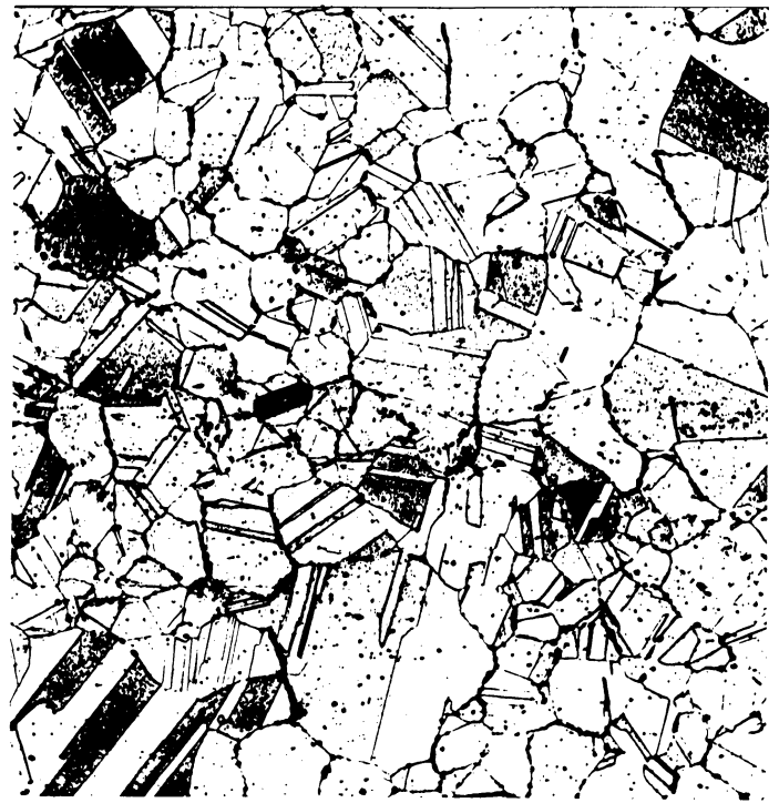
Figure 49 100x Spec. C2-62 Creep-Exposure 50 hours at 1600°F to 3.8% Deformation, NOT Tensile Tested
