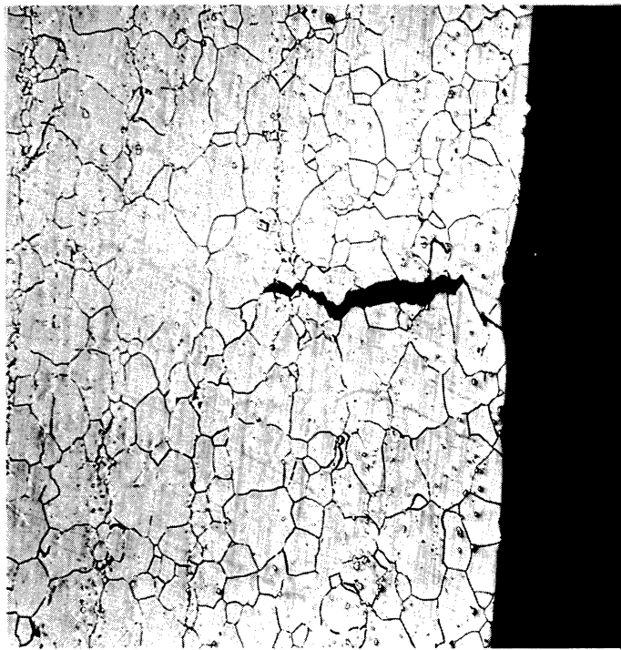
Fig. 8 Spec. No. R-95 (Section Showing Surface Attack and Isolated Crack) Creep-Exposure at 1300°F for 10 Hours to 2.71 Percent Deformation Subsequent Tensile Properties
