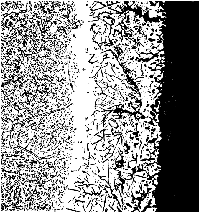
Fig. 7 Spec. No. D-2 (Section Showing Surface Attack) Exposed in Dilatometer Furnace 474 Hours at 1700°F
