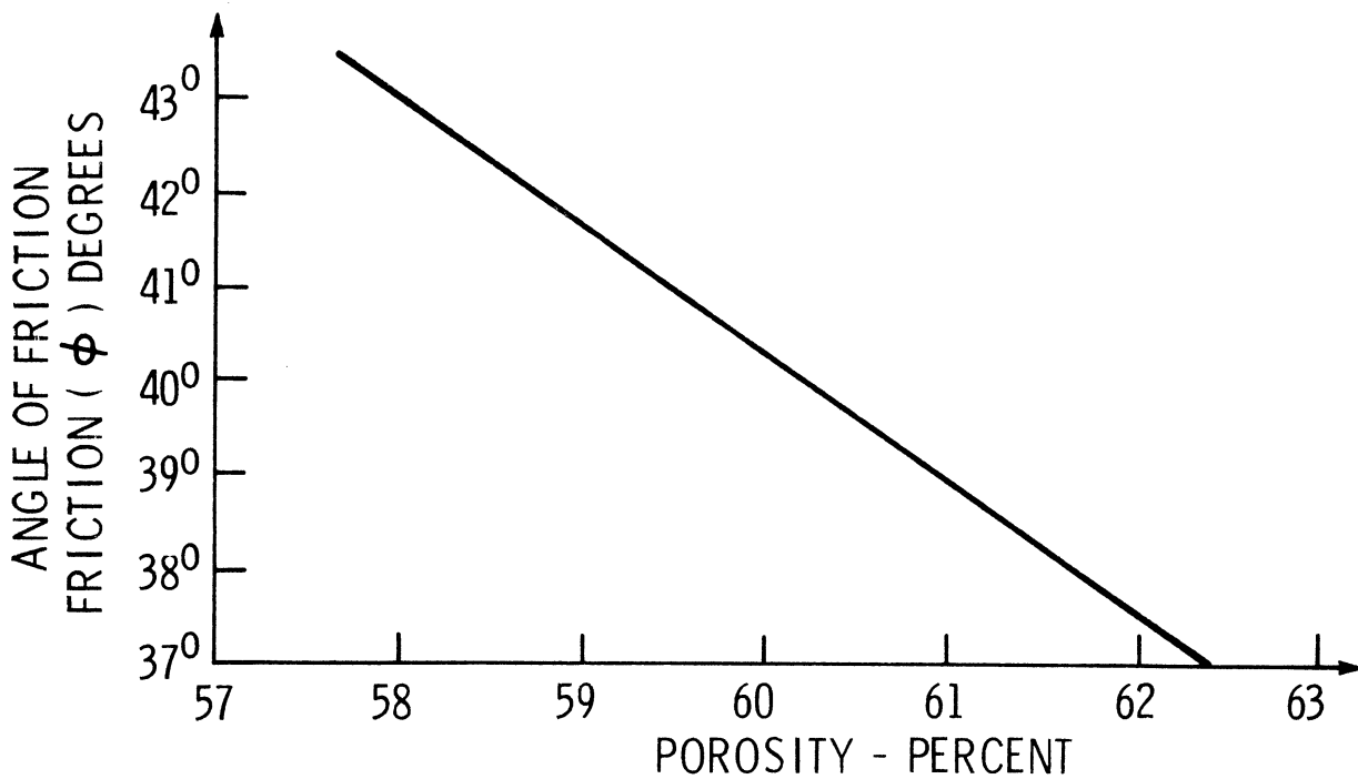
Figure 2. Effective angle of internal friction of ferrosilt-sand from Wilhemshaven, Germany (from Jenny, 1973)
