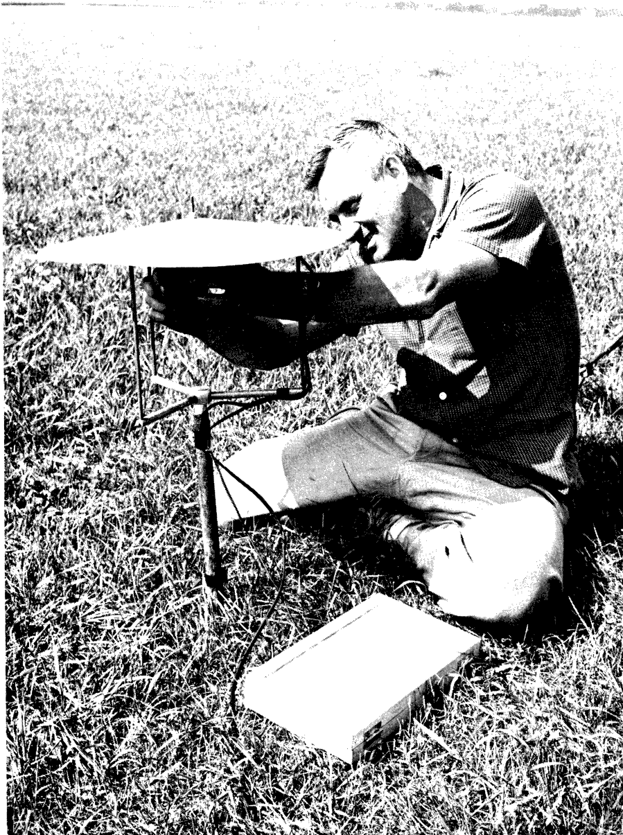
Fig. C.4. The rotobar sampler at 1/2 m above ground. The view is toward the north-west across Willow Run Airport. In-season experiment 1962.
