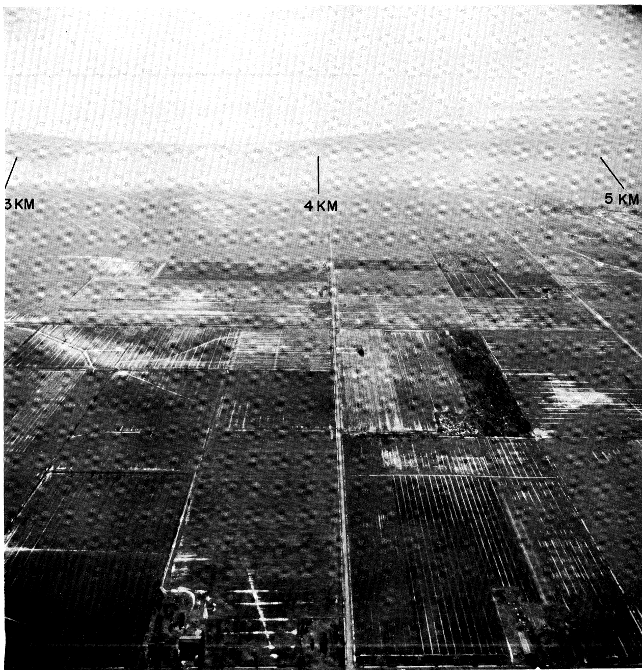
Fig. 13. Aerial view looking south, showing the greater diffusion of the smoke after an overland trajectory.
