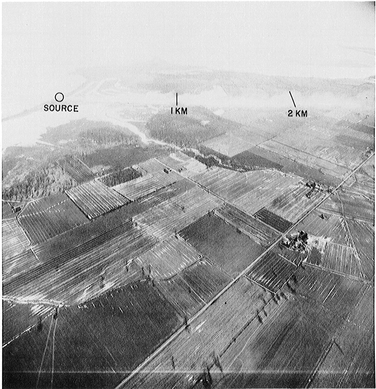
Fig. 11. Aerial view looking south as smoke leaves tower and flows westward over the land.
