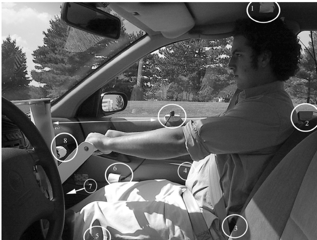
Figure 2. Interior of the vehicle. Circles highlight thermocouple and pyranometer positions.
